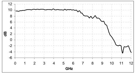
Figure 3: Frequency response of AMT8650-T46L-EVA (-20dBm optical input)
