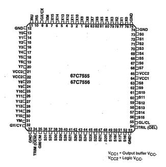
All VCC and GND pins must be connected to the respective VCC and GND connections on the board and should not be used for daisychaining through the IC.
