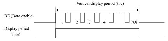
Note1: This diagram indicates virtual signal for set up to timing.
