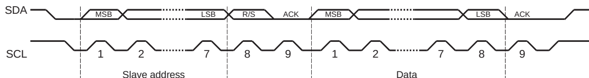
Figure 14-5. Complete Data Transfer with a 7-Bit Address
