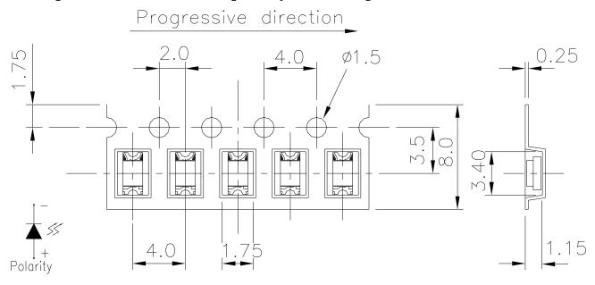
**Note:** Tolerances Unless Dimension ±0.1mm, Unit = mm
