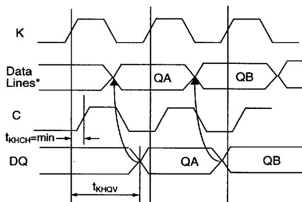
**Dual Clock Diagram #2:** Internal data lines await at the output latch for the rising edge of C clock. The C clock enables the output latch and allows output data to become available.
