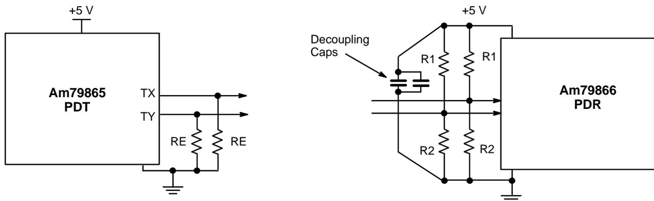
**Figure 3. Decoupling Terminations**
