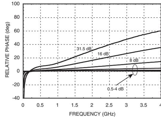
**0.5 dB LSB GaAs MMIC 6-BIT DIGITAL POSITIVE CONTROL ATTENUATOR, DC - 3.0 GHz**
