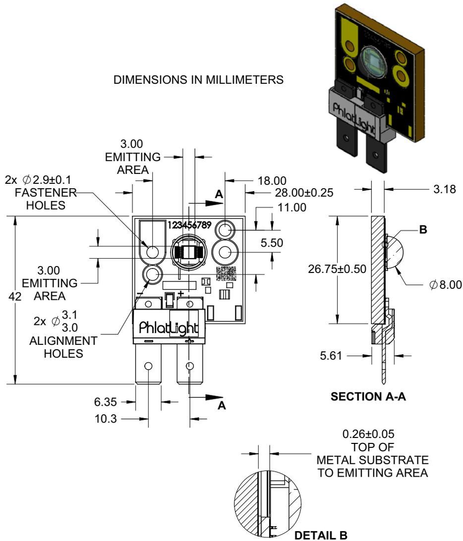
Recommended connector for Anode and Cathode: Panduit Disco Lok™ Series P/N: DNG14-250FL-C
