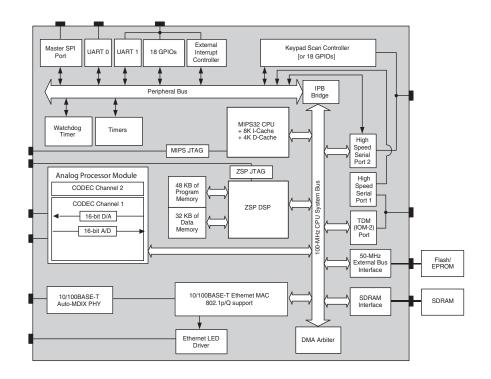
Broadcom's BCM1115R is designed for use in feature-reduced, costsensitive, single Ethernet port consumer and Enterprise IP Phone and Gateway products.
