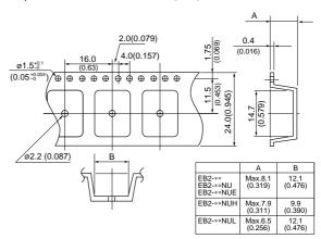
Relay orientation mark and tape carrying direction.
