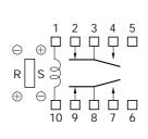
Single coil latch type (reset position)
