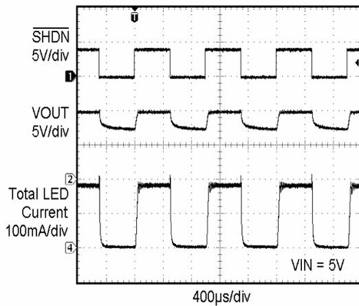
Figure 1. Switching Waveform with 1kHz PWM on SHDN
