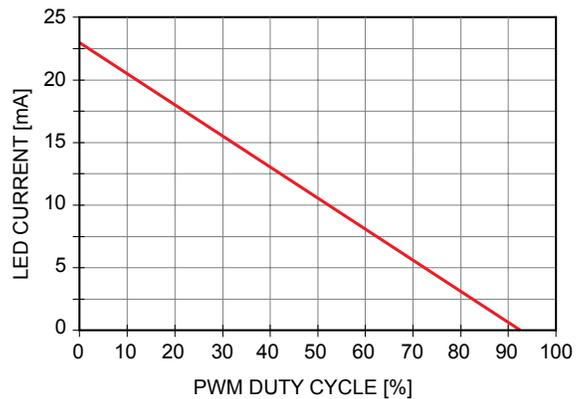
Figure 3. Filtered PWM Dimming [0V to 2.5V]
