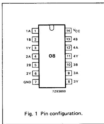
Fig. 1 Pin configuration.
