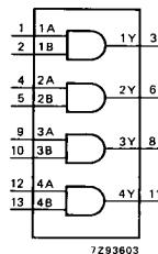
Fig. 4 Functional diagram.
