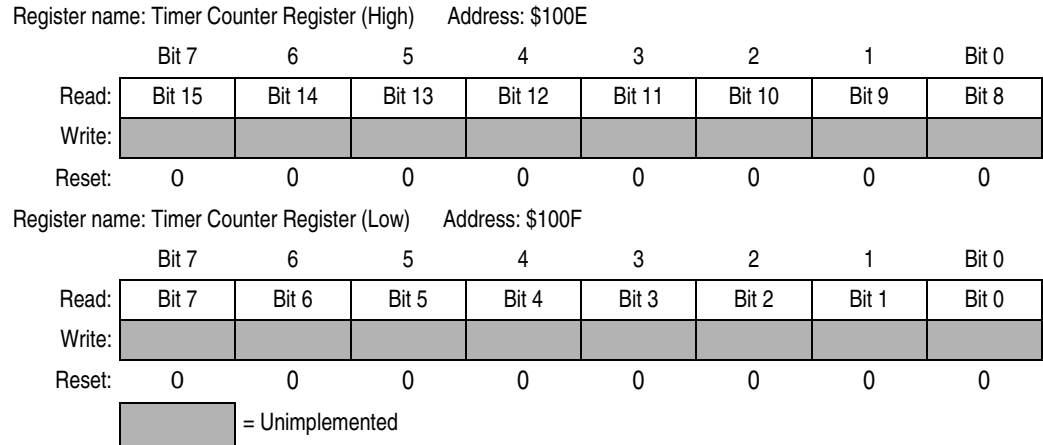
Figure 9-15. Timer Counter Register (TCNT)
