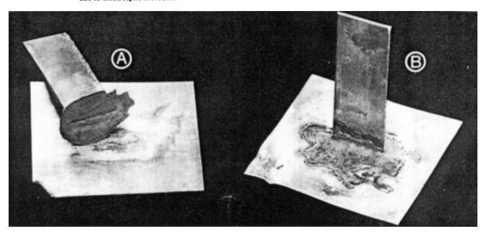
designed so that the solder is subjected only to shear stresses. Joint clearances should be 0.05-0.10 mm for best strength and capillary effect.
