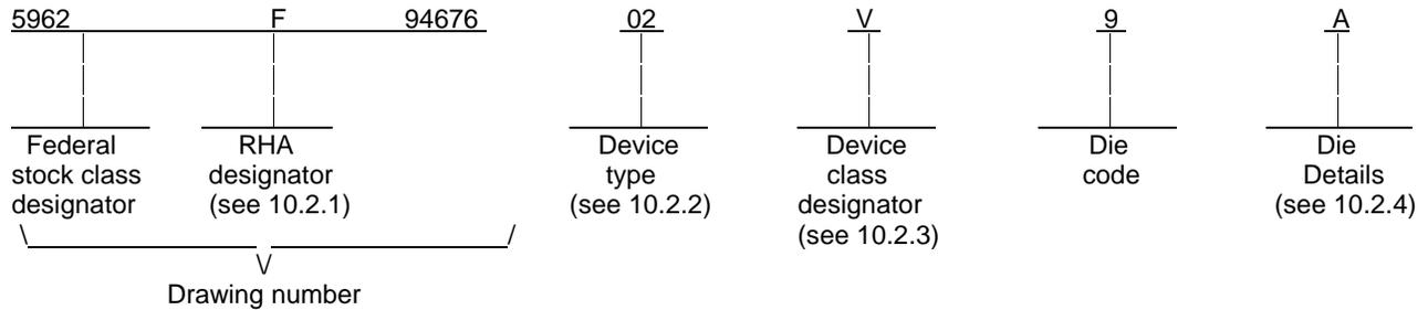
10.2.1 RHA designator. Device classes Q and V RHA identified die shall meet the MIL-PRF-38535 specified RHA levels. A dash (-) indicates a non-RHA die.
