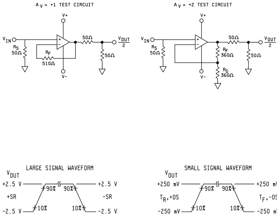
FIGURE 2. Test circuits and waveforms - Continued.
