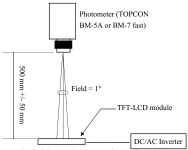
Optical characteristics measuring configuration
