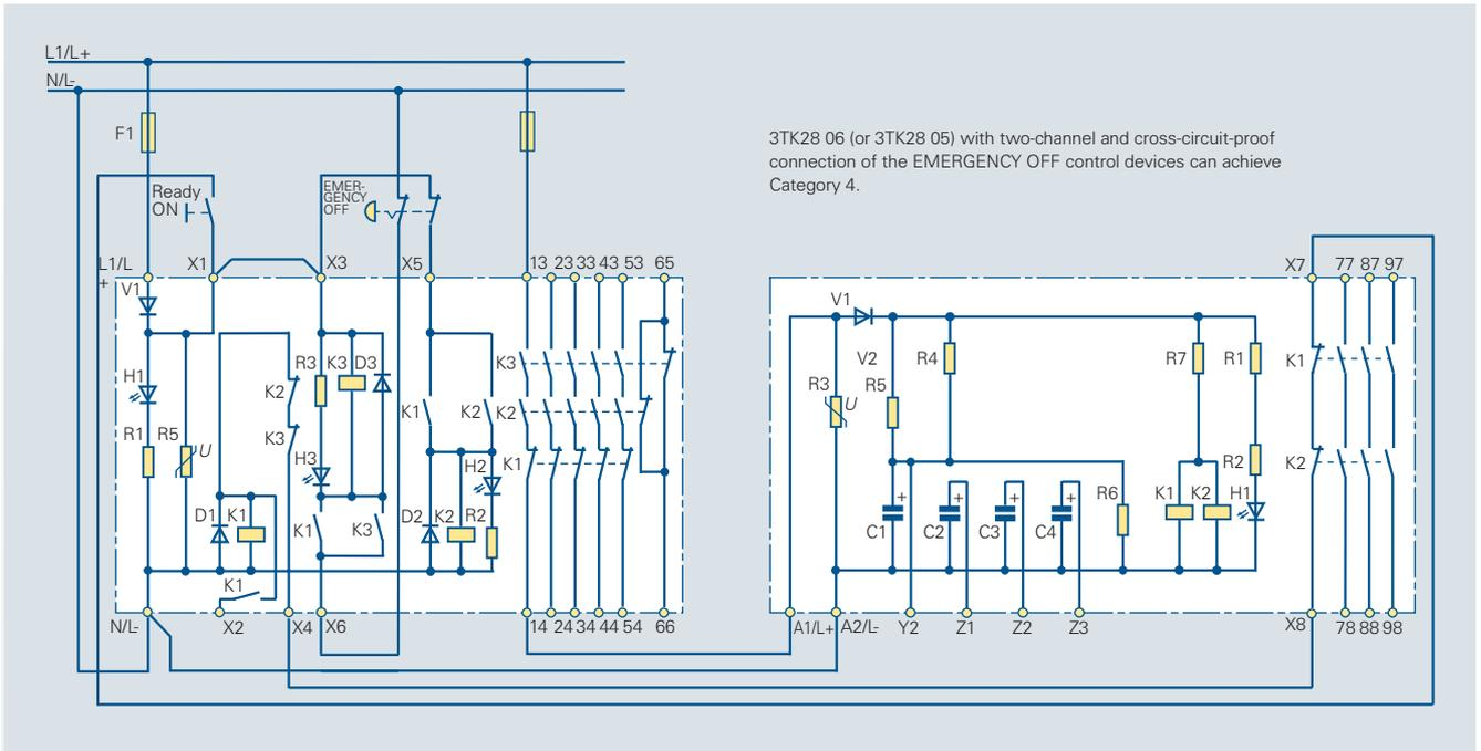
3TK28 06 (or 3TK28 05) with two-channel and cross-circuit-proof connection of the EMERGENCY OFF control devices can achieve Category 4.
