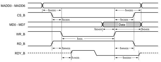
c) Internal register read/write (NEASCOT-S15 connection mode, MSEL = "0")
