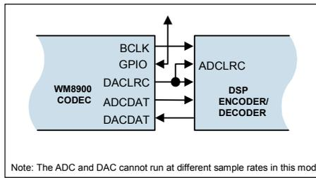
Figure 27 Master Mode with ADCLRC as GPIO
