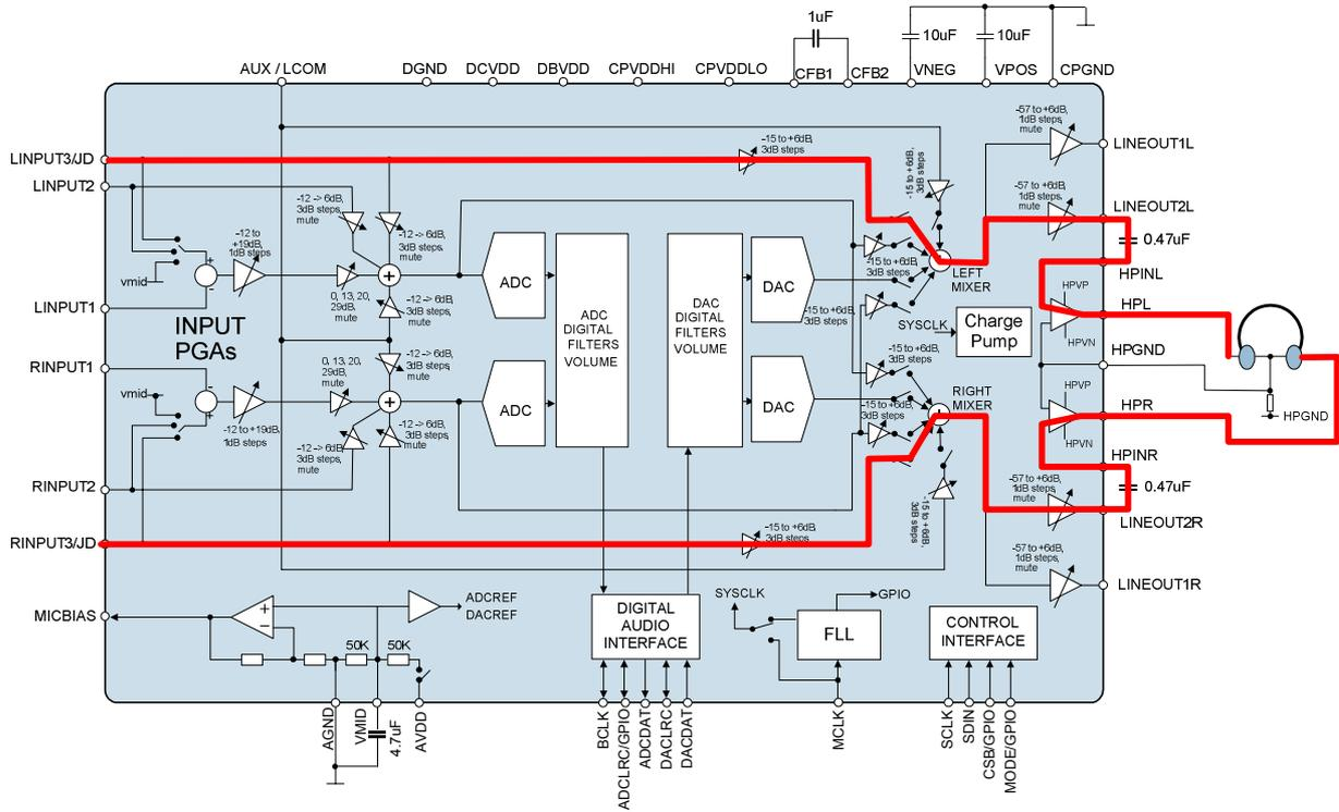
**Figure 66 LR Input 3 to Headphone Bypass Path**
