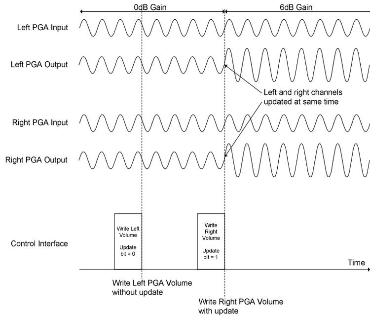
**Figure 21 Simultaneous Left and Right Volume Updates**
