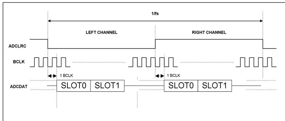
Figure 41 TDM in I<sup>2</sup>S Mode
