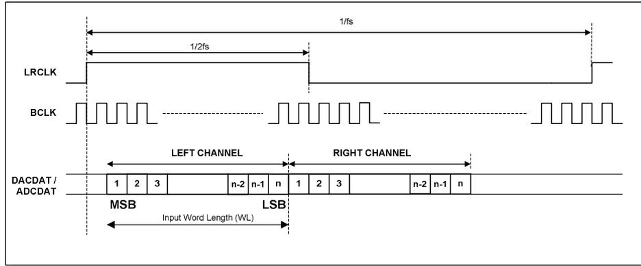
Figure 35 DSP/PCM Mode Audio Interface (mode A, AIF\_LRCLKINV=0, Master)
