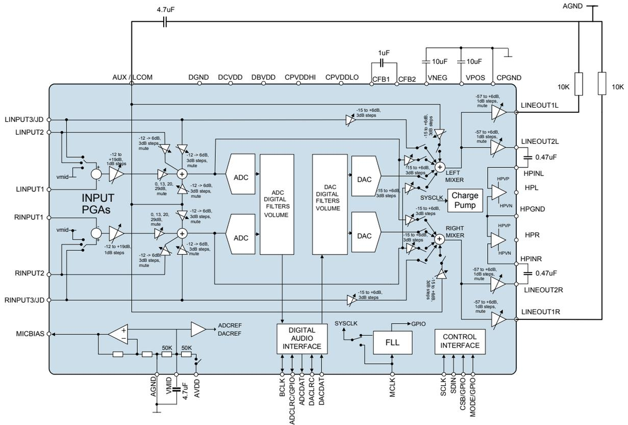
Figure 19 LCOM Common Ground Connection for LINEOUT1
