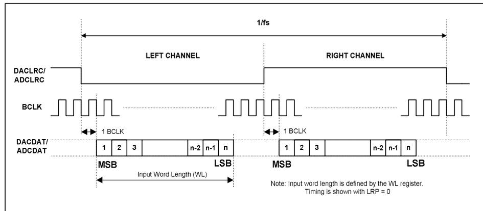
Figure 34 I<sup>2</sup>S Justified Audio Interface (assuming n-bit word length)
