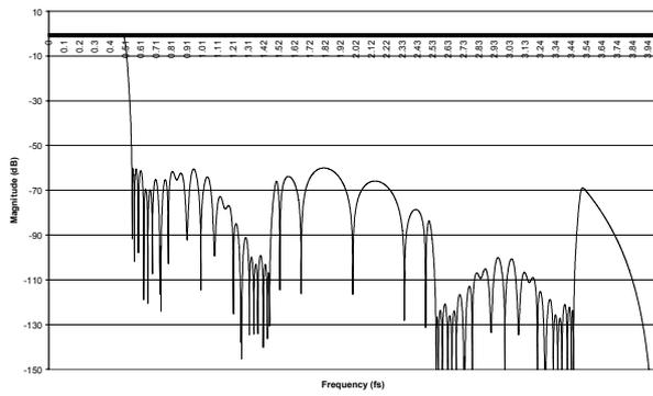
Figure 50 ADC Digital Filter Frequency Response
