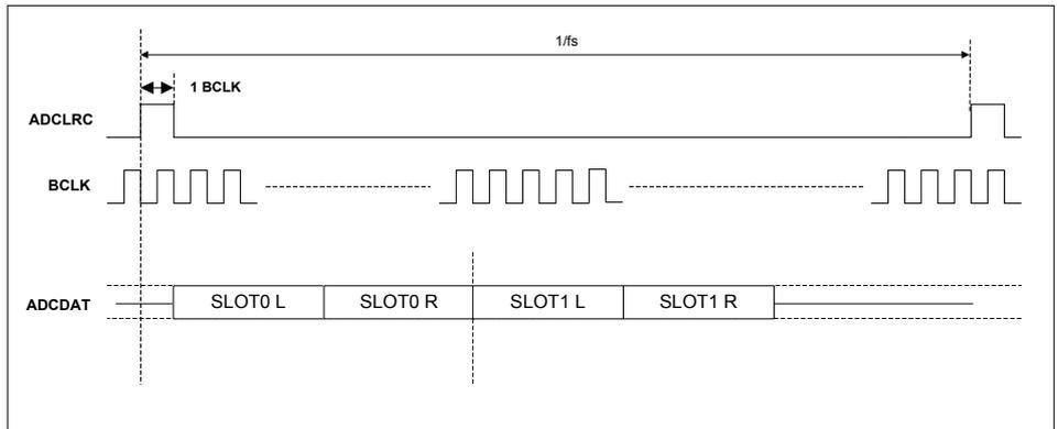
Figure 42 TDM in DSP/PCM Mode A
