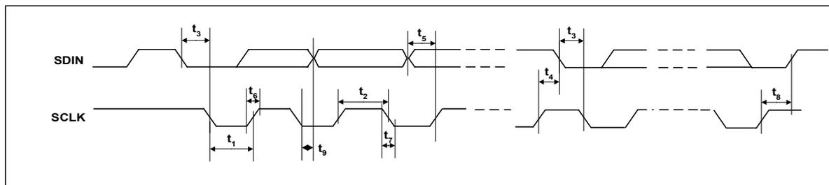
Figure 7 Control Interface Timing – 2-Wire Serial Control Mode
