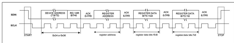
**Figure 48 2-Wire Serial Control Interface Writes**
