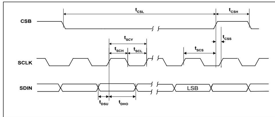
Figure 8 Control Interface Timing – 3-Wire Serial Control Mode
