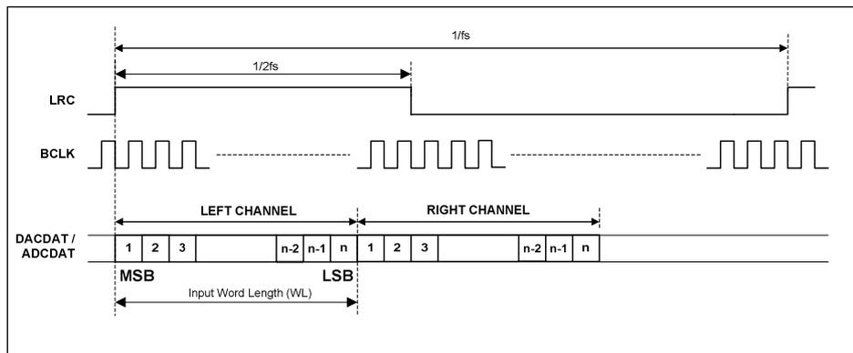
Figure 36 DSP/PCM Mode Audio Interface (mode B, AIF\_LRCLKINV =0, Master)
