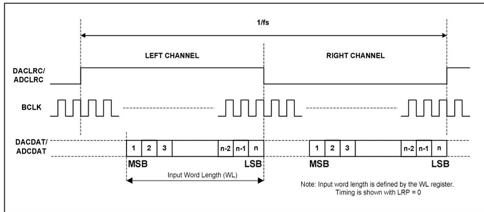
Figure 33 Right Justified Audio Interface (assuming n-bit word length)
