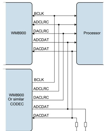
Figure 30 TDM with Other CODEC as Master
