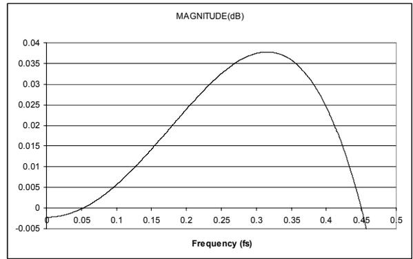
Figure 53 DAC Digital Filter Ripple (Normal Mode)
