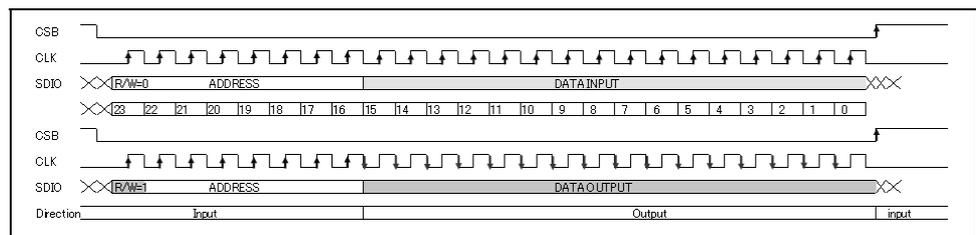
**Figure 47 3-Wire Serial Control Timing**
