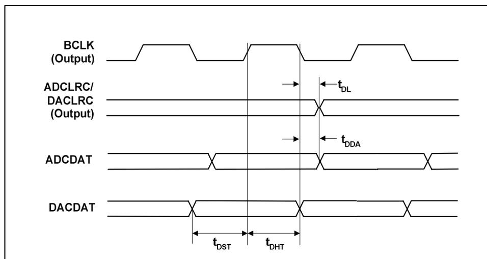
Figure 5 Digital Audio Data Timing - Master Mode
