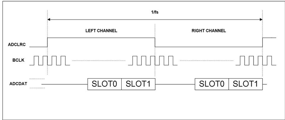
Figure 40 TDM in Right-Justified Mode
