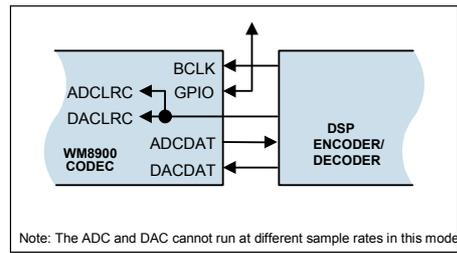
Figure 28 Slave Mode with ADCLRC as GPIO
