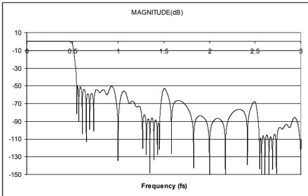
Figure 52 DAC Digital Filter Frequency Response (Normal Mode)
