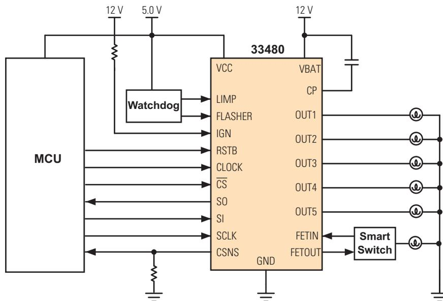
Figure 1. 33480 Simplified Application Diagram
