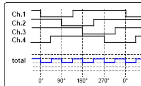
The synchronization of the switching phases between different corner light IC is provided by an SPI command in combination with the CS input. The bit in the SPI is called PWM sync (initialization register).
