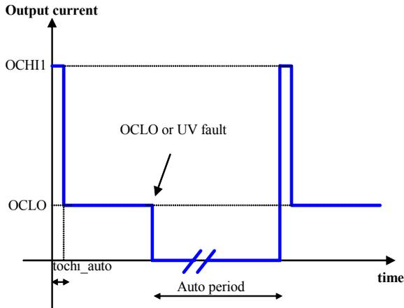
**Figure 7. Overcurrent window in case of Autorestart**
