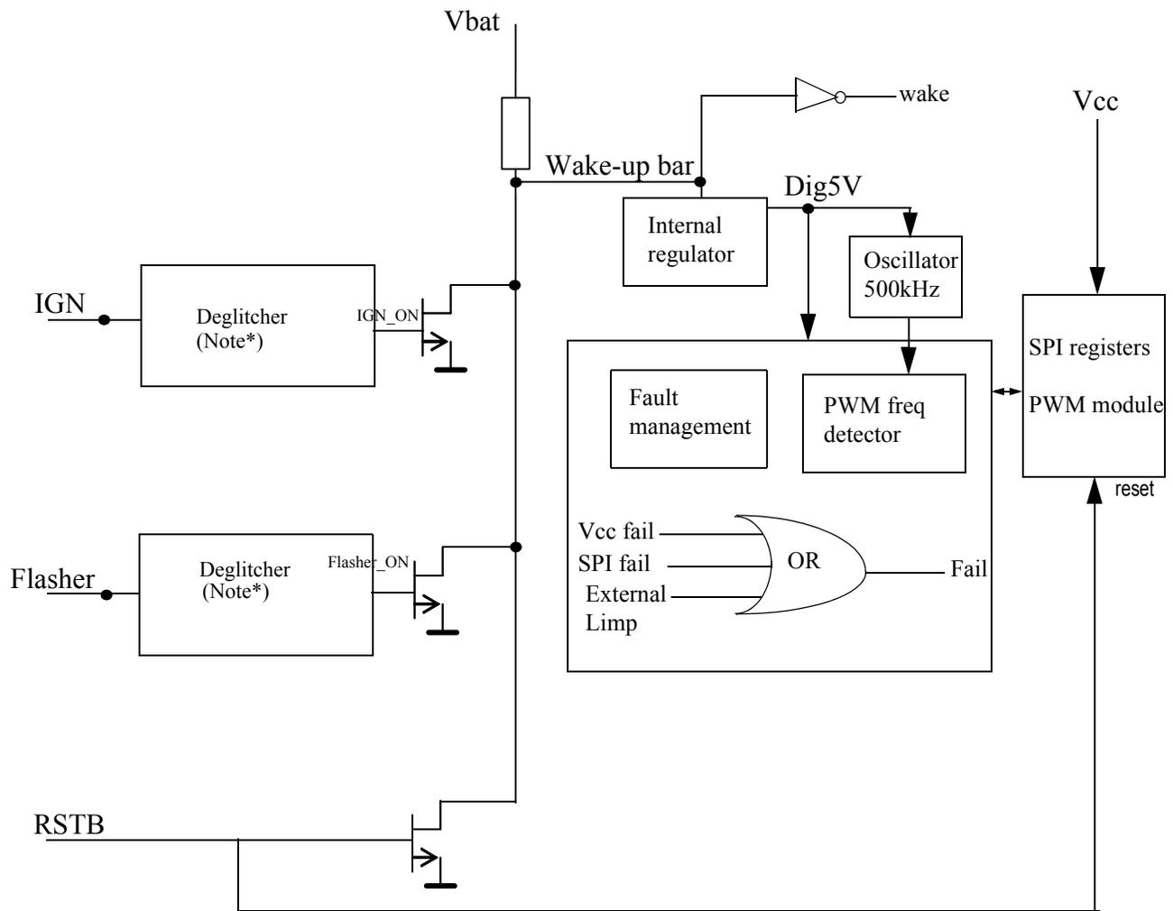
Figure 9. Wake-up block diagram
