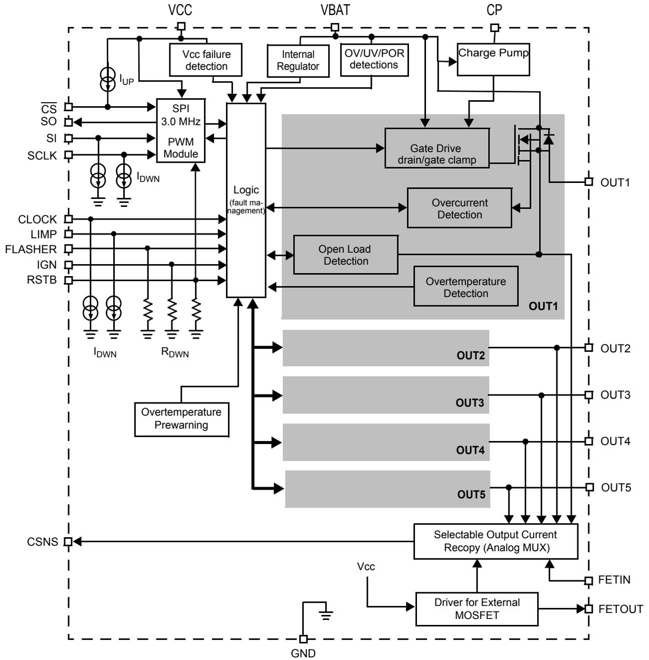
Figure 2. 33480 Simplified Internal Block Diagram
