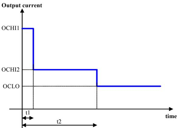
Figure 10. Double overcurrent window in Normal Mode
