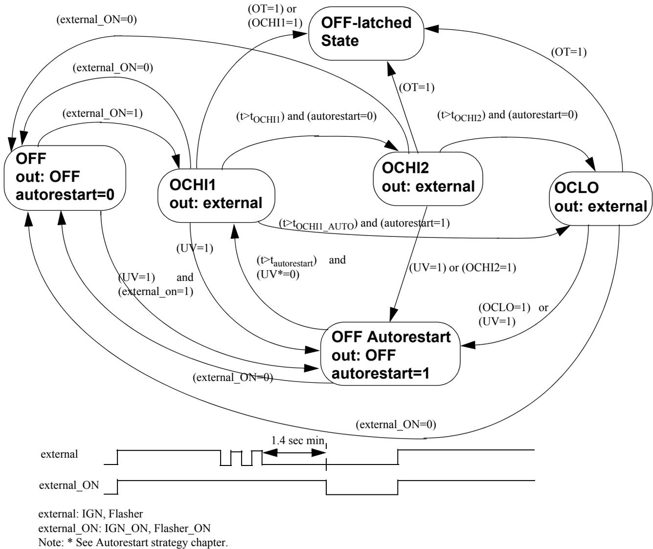
Figure 12. Faults management in Fail Mode (for OUT[1:5] only)
