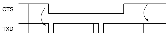
Figure 21-28. Transmitter Behavior when Operating with Hardware Handshaking
