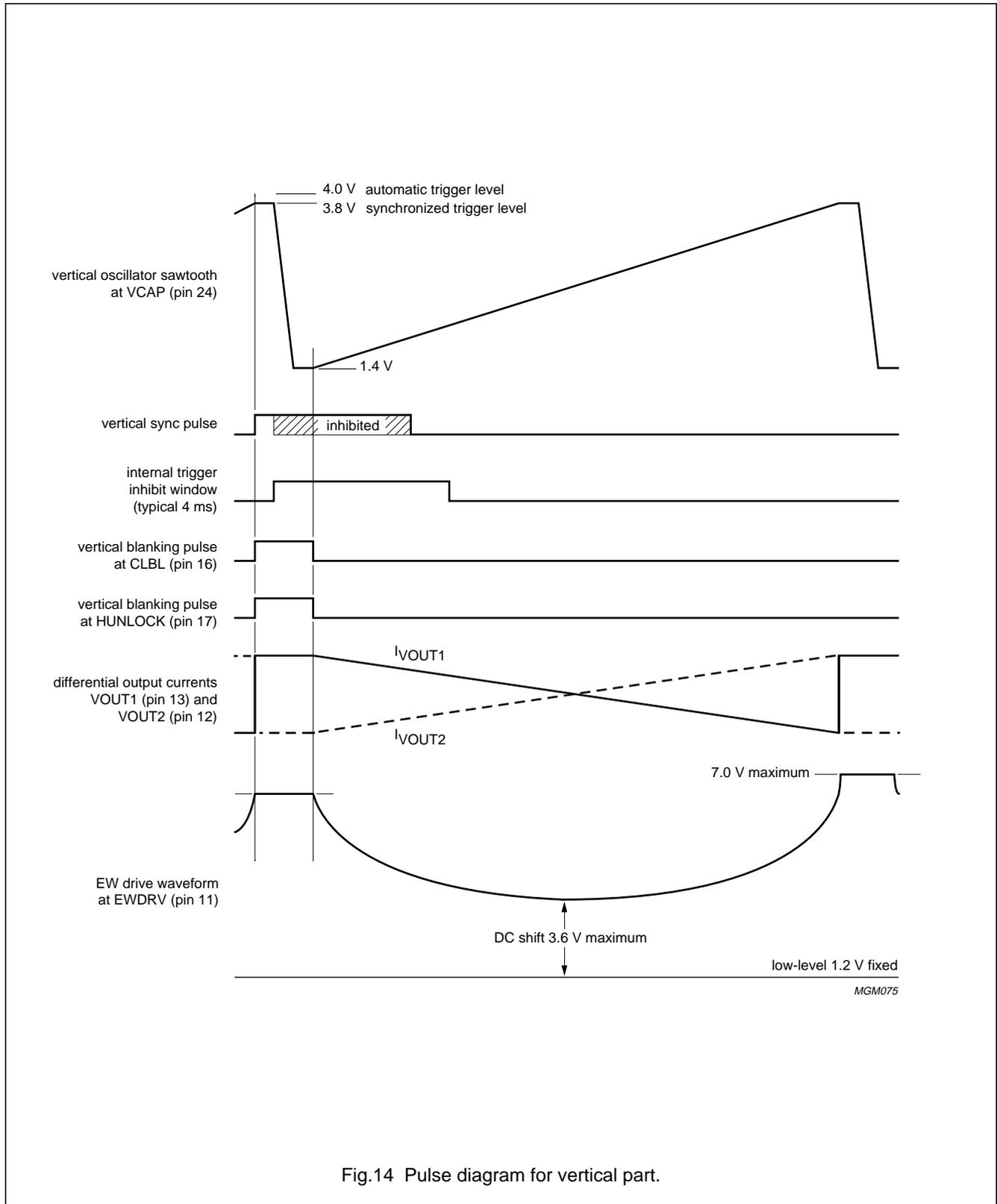
Fig.14 Pulse diagram for vertical part.
