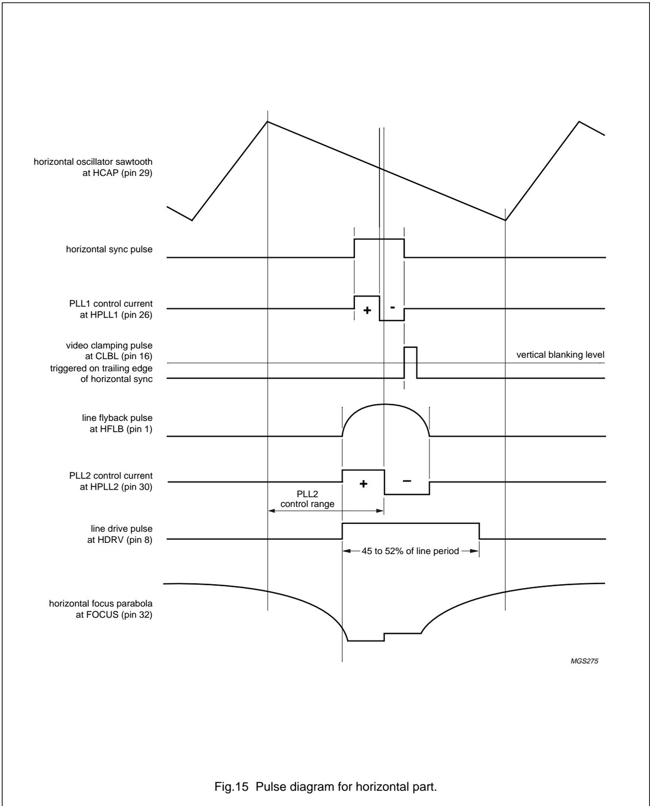
Fig.15 Pulse diagram for horizontal part.
