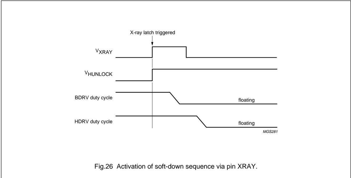
Fig.26 Activation of soft-down sequence via pin XRAY.
