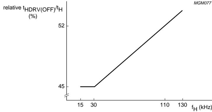
Fig.16 Relative t<sub>OFF</sub> time of HDRV versus H-frequency.
