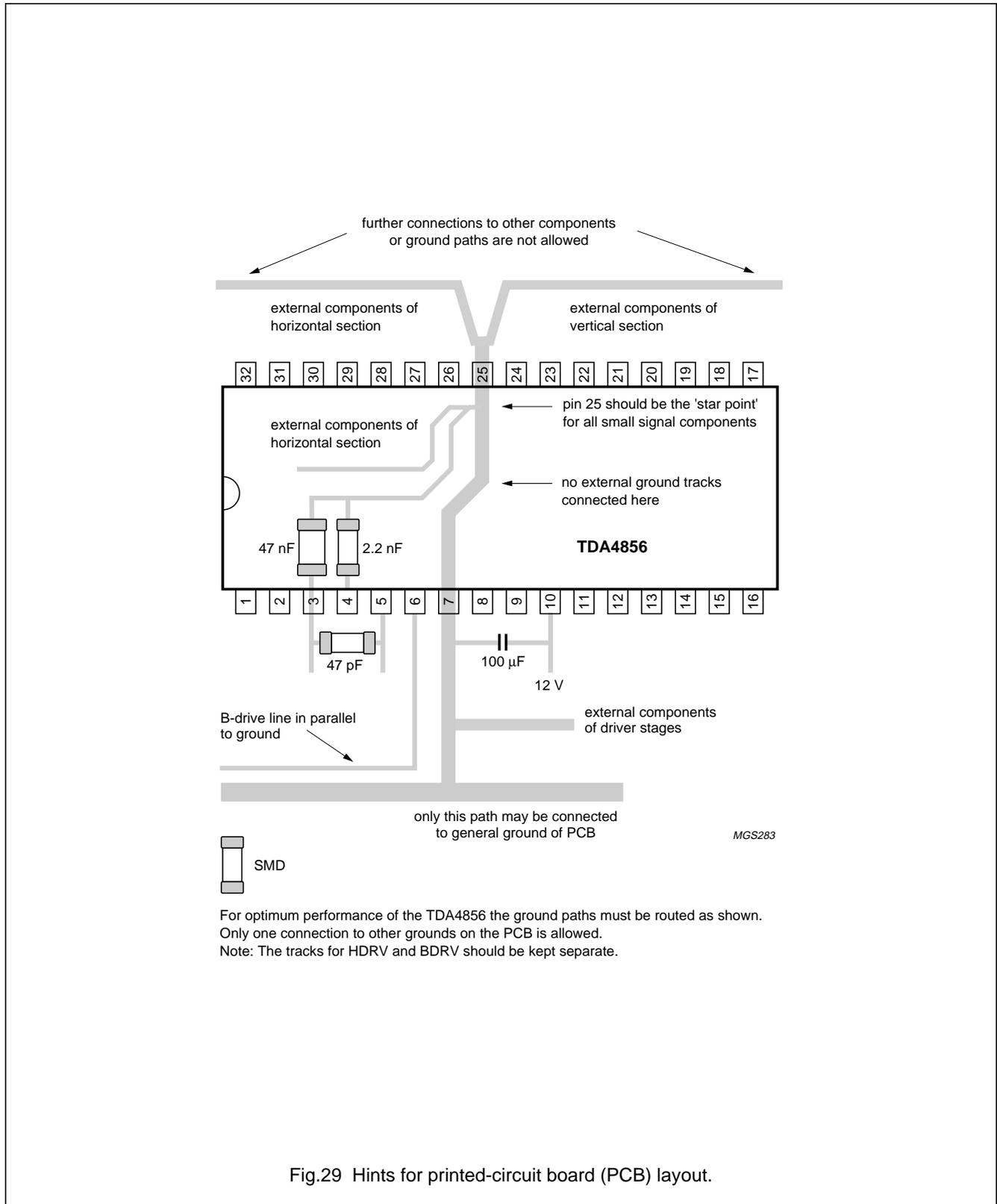
Fig.29 Hints for printed-circuit board (PCB) layout.
