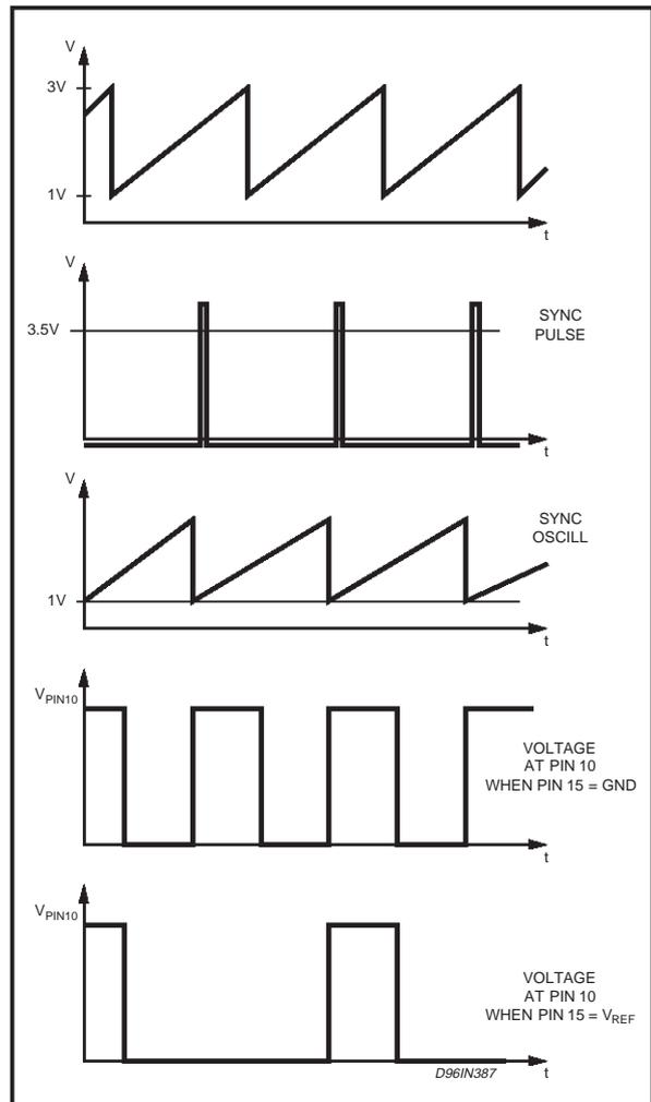
The oscillator can be synchronised by a voltage pulse sent to pin1.
