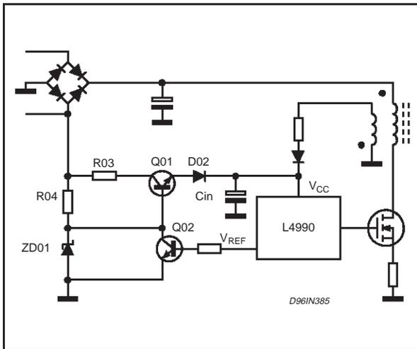
Fig2-a is well suited to applications with fixed mains, 110 or 220Vac; it's the cheapest and largely used system to start-up an IC with hysteretic turn-on.
