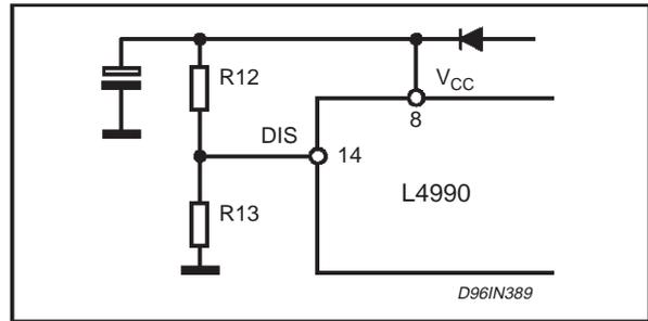
monitor the auxiliary supply through R12 and R13.
