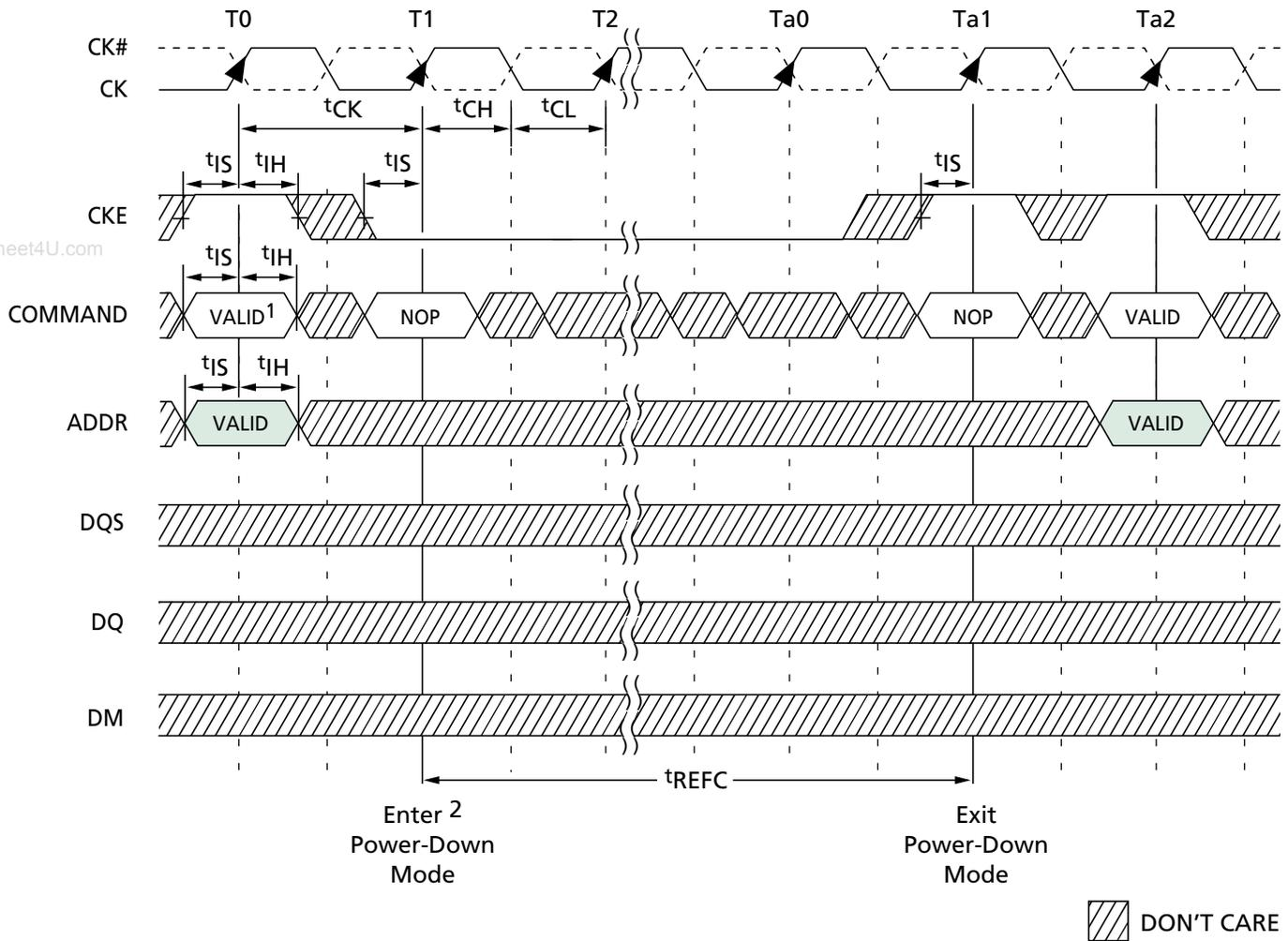
**NOTE:** 1. If this command is a PRECHARGE (or if the device is already in the idle state), then the power-down mode shown is precharge power-down. If this command is an ACTIVE (or if at least one row is already active), then the power-down mode shown is active power-down.
