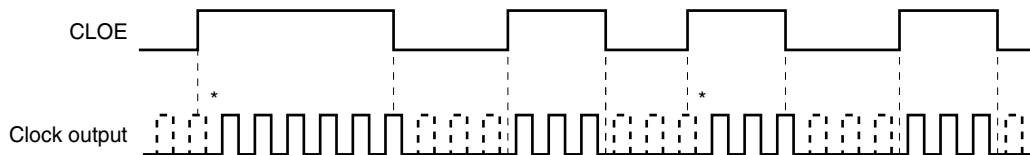
Figure 11-4. Remote Control Output Application Example
