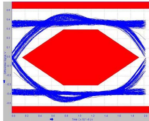
Figure 6. Audio Switch Near End Eye Diagram (V<sub>CC</sub> = 3.6 V, IN1 = 1, IN2 = 0, Temp = 25°C)
