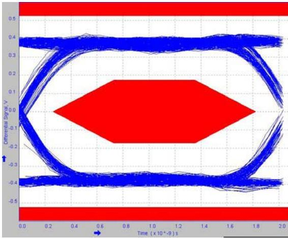
**Figure 7. Reference Far End Eye Diagram**
