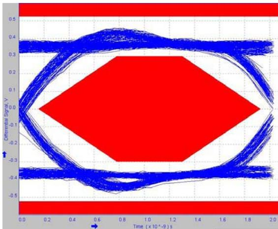
Figure 5. UART Switch Near End Eye Diagram (V<sub>CC</sub> = 3.6 V, IN1 = 1, IN2 = 1, Temp = 25°C)
