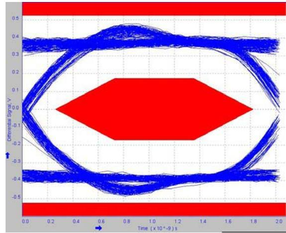
**Figure 10. Audio Switch Far End Eye Diagram**
