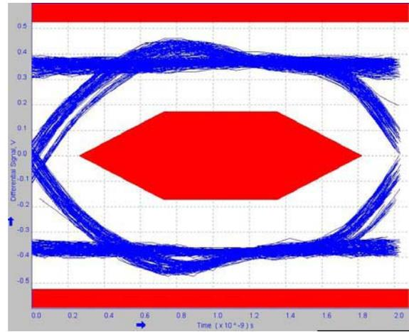
**Figure 8. USB Switch Far End Eye Diagram**
