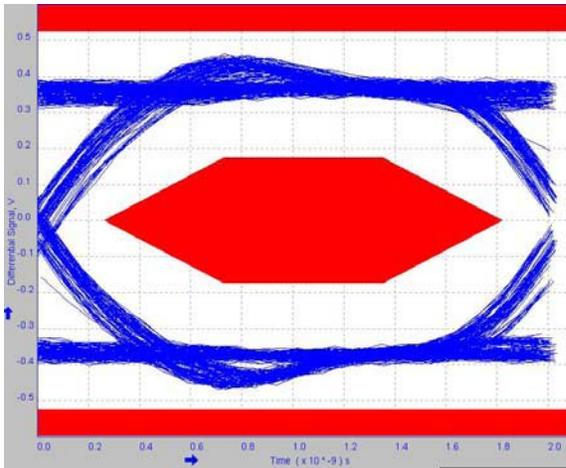
**Figure 9. UART Switch Far End Eye Diagram**
