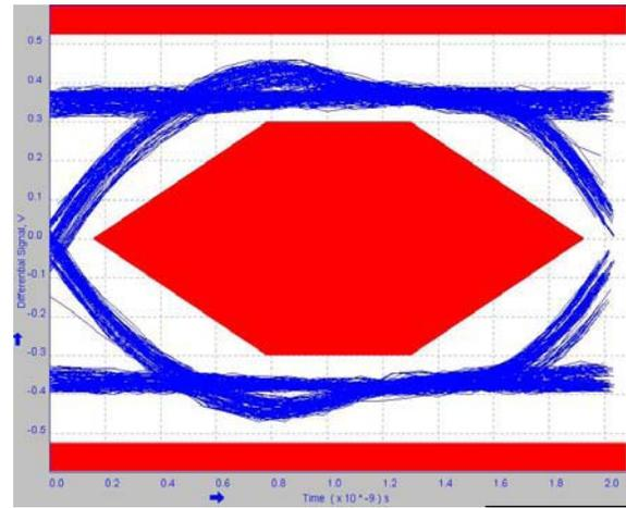
Figure 4. USB Switch Near End Eye Diagram (V<sub>CC</sub> = 3.6 V, IN1 = 0, IN2 = 1, Temp = 25°C)
