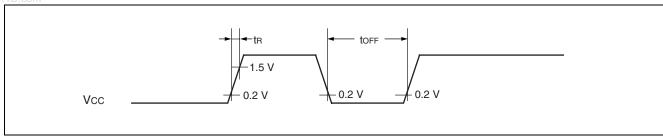
Note: Sudden change of power supply voltage may activate the power-on reset function. When changing power supply voltages during operation, set the slope of rising within 20 mV/ms as shown below.
