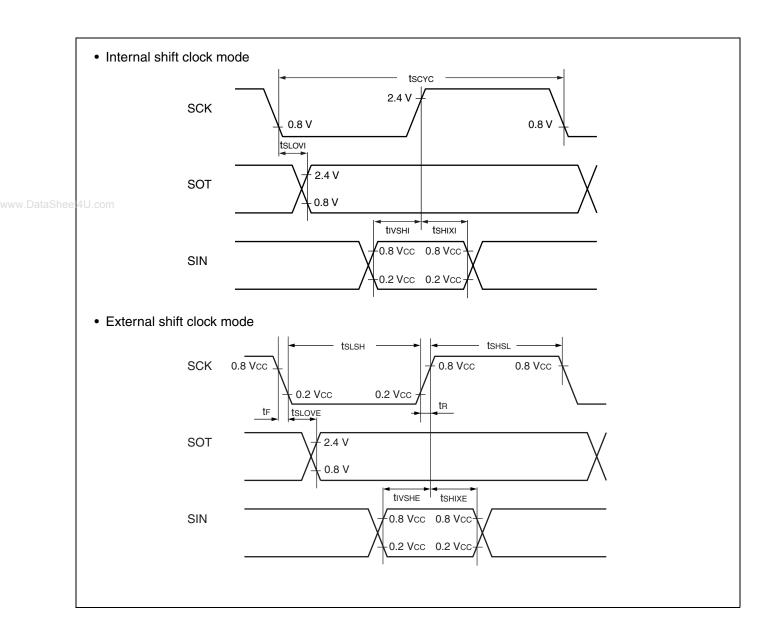
Sampling at the falling edge of sampling clock\*1 and prohibited serial clock delay\*2 (ESCR register : SCES bit = 1, ECCR register : SCDE bit = 0)
