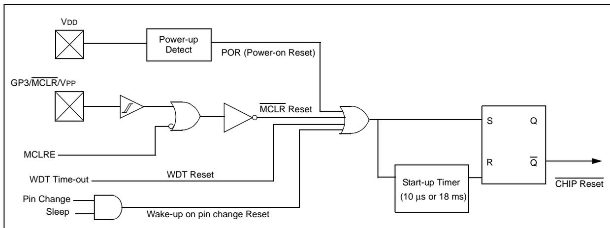
**FIGURE 9-3: TIME-OUT SEQUENCE ON POWER-UP ( $\overline{\text{MCLR}}$  PULLED LOW)**
