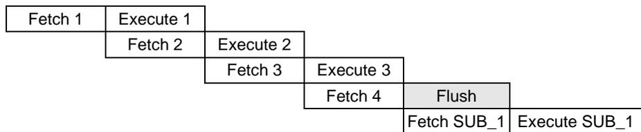
All instructions are single cycle, except for any program branches. These take two cycles, since the fetch instruction is "flushed" from the pipeline, while the new instruction is being fetched and then executed.
