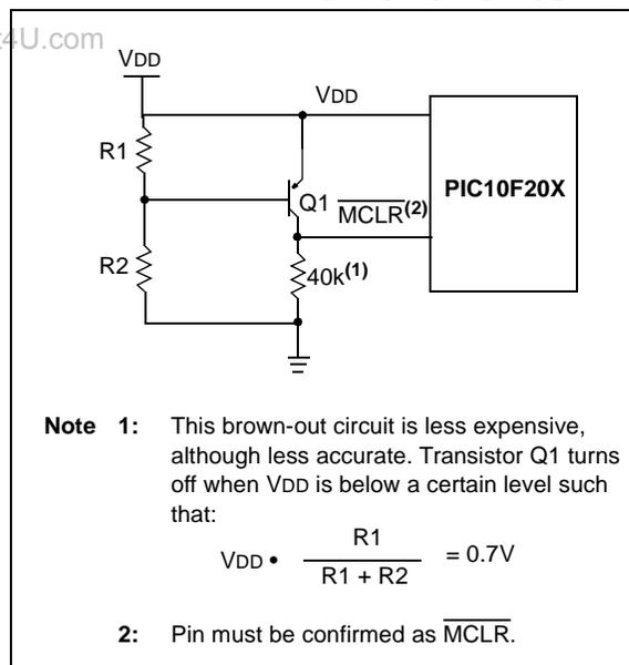
**FIGURE 9-9: BROWN-OUT PROTECTION CIRCUIT 3**
