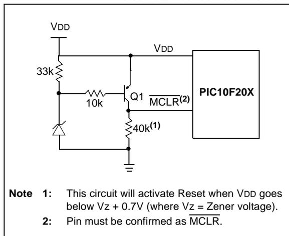
**FIGURE 9-8: BROWN-OUT PROTECTION CIRCUIT 2**
