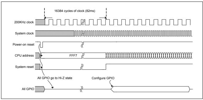
Figure 5-4 Power-up procedure
