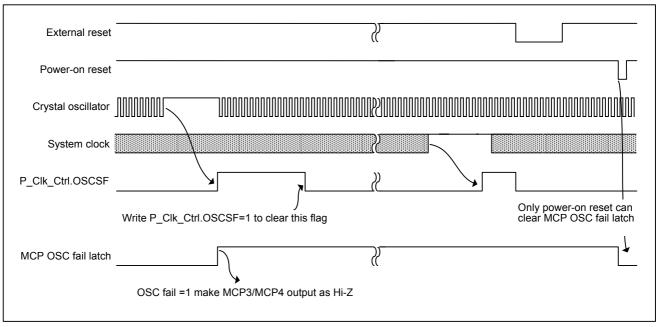
Figure 5-8 Clock Fail timing
