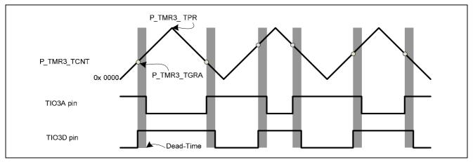
Figure 5-64 Active-low PWM mode of dead-time generation
