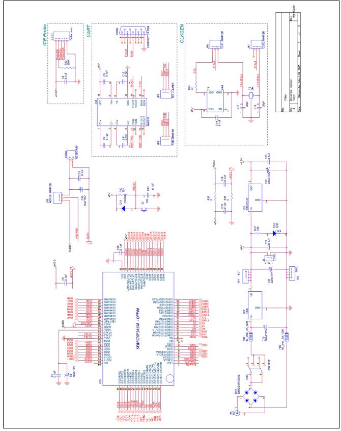
Figure 7-1 SPMC75F2413A EVM board circuit part I
