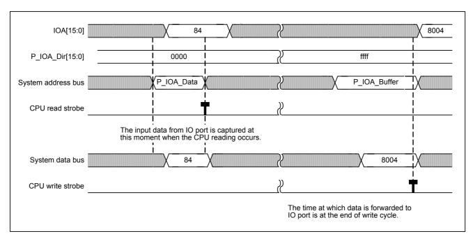
Figure 5-20 GPIO input/output timing
