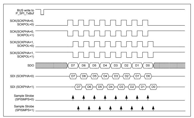
Figure 5-73 SPI mode timing, Master Mode
