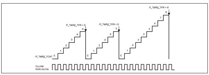
Figure 5-43 Continuous up counting example (CCLS = 111'b, CKEGS = 00'b, TMRPS = 000'b)
