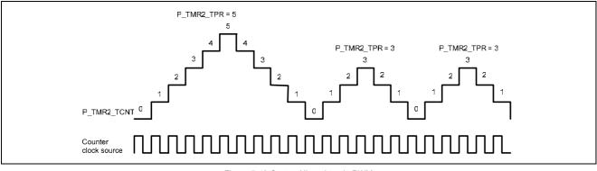
Figure 5-49 Center-Aligned mode PWM
