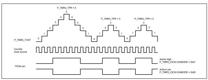
Figure 5-58 Center-Aligned mode PWM
