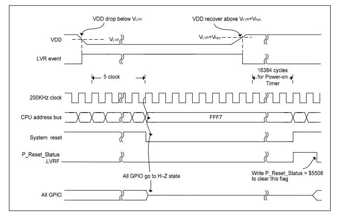
Figure 5-15 Low voltage reset timing
