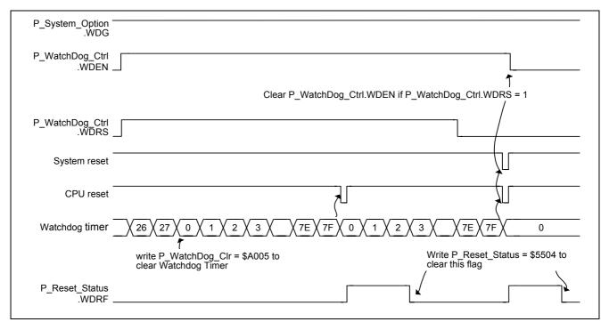
Figure 5-86 Watchdog Timing Diagram
