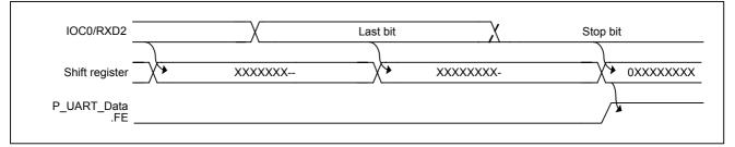
Figure 5-82 Frame Error timing
