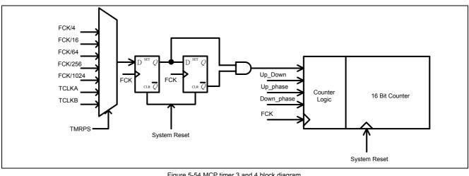
Figure 5-54 MCP timer 3 and 4 block diagram
