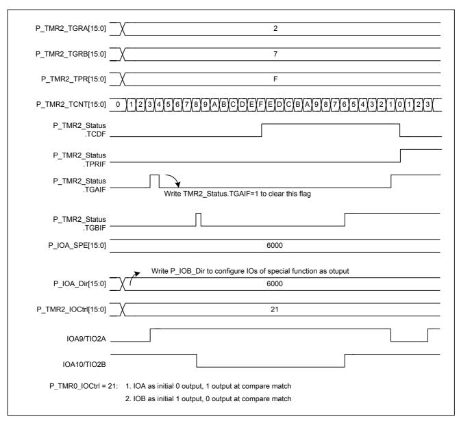
Figure 5-50 TMR2 center aligned PWM
