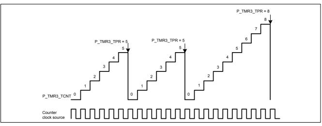
Figure 5-55 Continuous up counting example (CCLS = 111'b, CKEGS = 00'b, TMRPS = 000'b)
