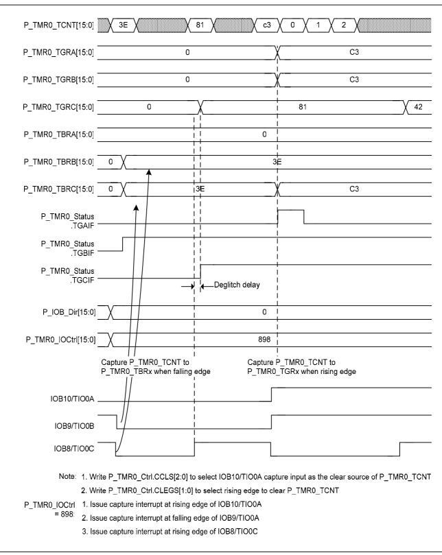
Figure 5-34 Capture input signal width and cycle
