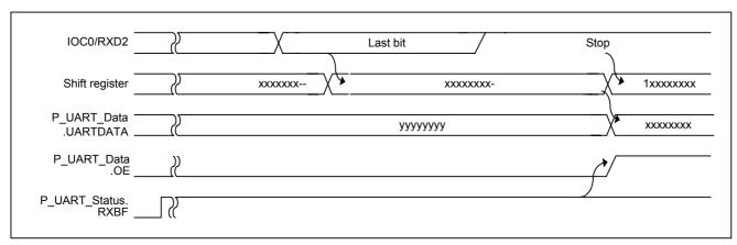
Figure 5-80 Overrun error timing
