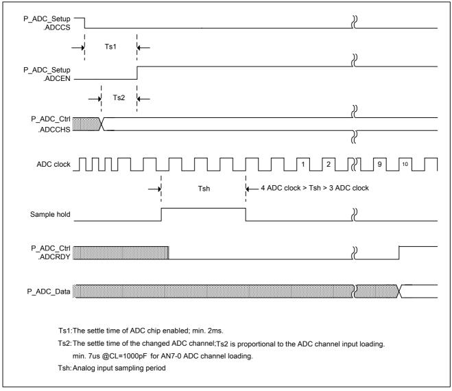
Figure 5-84 ADC timing diagram
