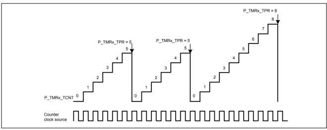
Figure 5-23 Continuous up counting example (CCLS = 111'b, CKEGS = 00'b, TMRPS = 000'b)
