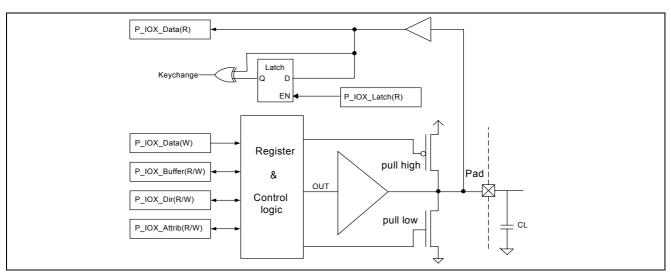
Figure 5-19 IO structure diagram
