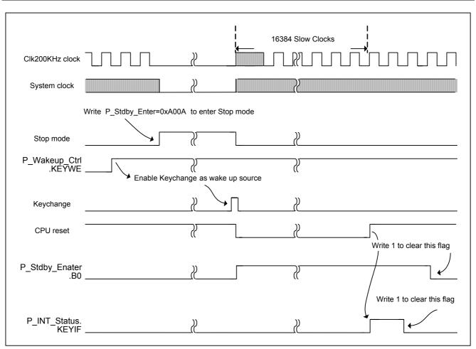
Figure 5-10 Standby mode timing
