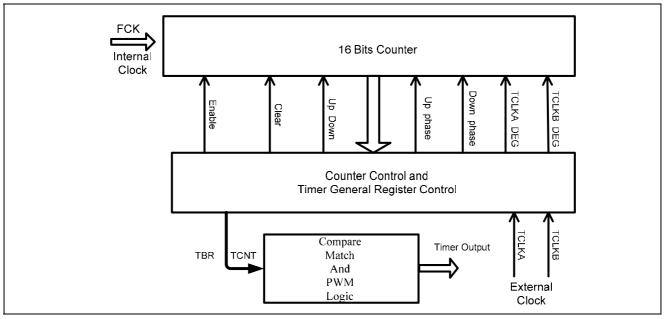
Figure 5-42 TPM timer 2 block diagram
