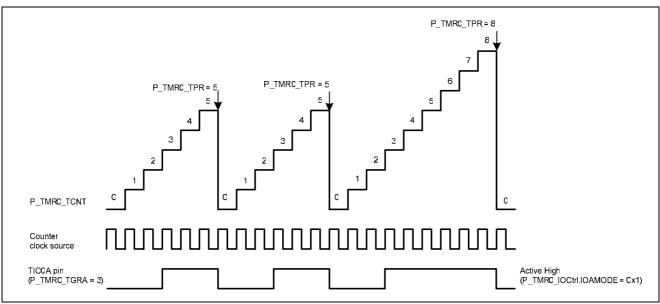
Figure 5-25 Edge-Aligned mode PWM
