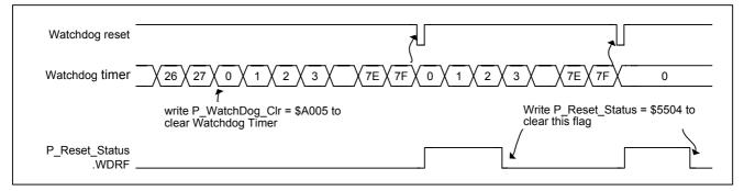
Figure 5-16 Watchdog timer reset timing
