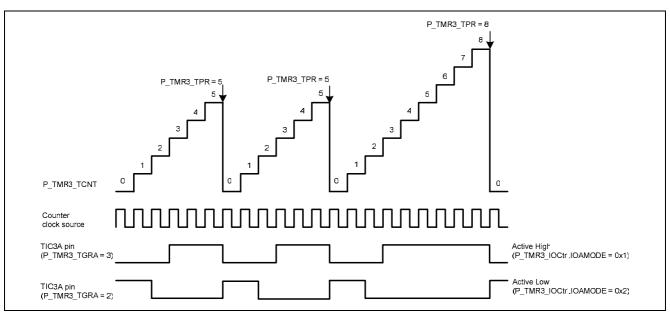
Figure 5-56 Edge-Aligned mode PWM
