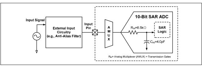
Figure 5-83 ADC equivalent circuit for SPMC75F2413A
