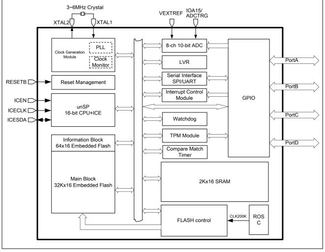
Figure 3-1 SPMC75F2413A function block diagram
