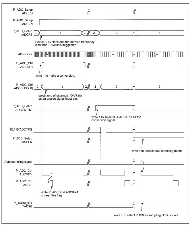
Figure 5-85 AD conversion timing
