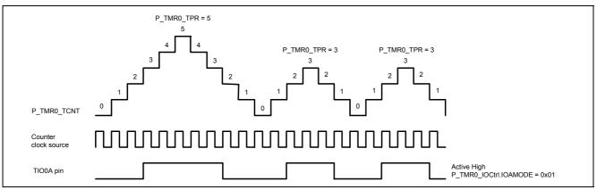
Figure 5-30 Center-aligned mode PWM
