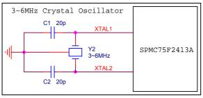
Figure 5-5 The crystal circuit connection
