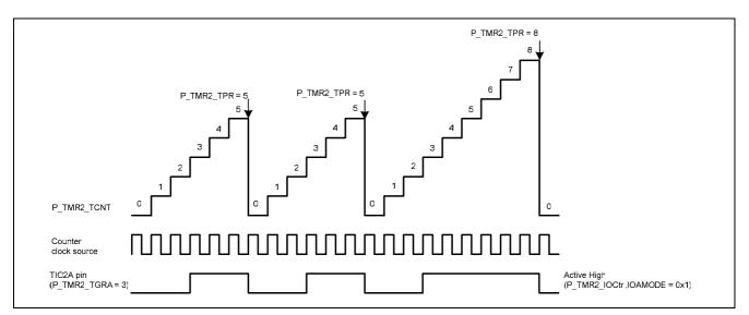
Figure 5-44 Edge-Aligned mode PWM
