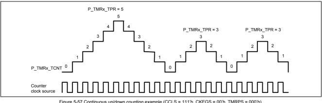
Figure 5-57 Continuous up/down counting example (CCLS = 111'b, CKEGS = 00'b, TMRPS = 000'b)
