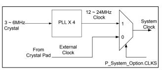
Figure 5-6 PLL and external clock block diagram
