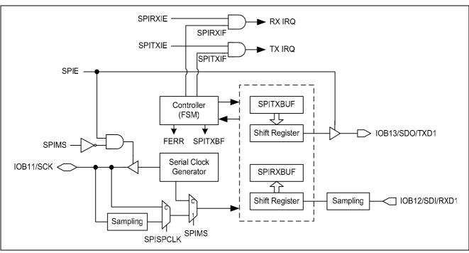
Figure 5-72 Function block diagram of SPI interface
