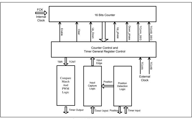
Figure 5-22 PDC timers block diagram
