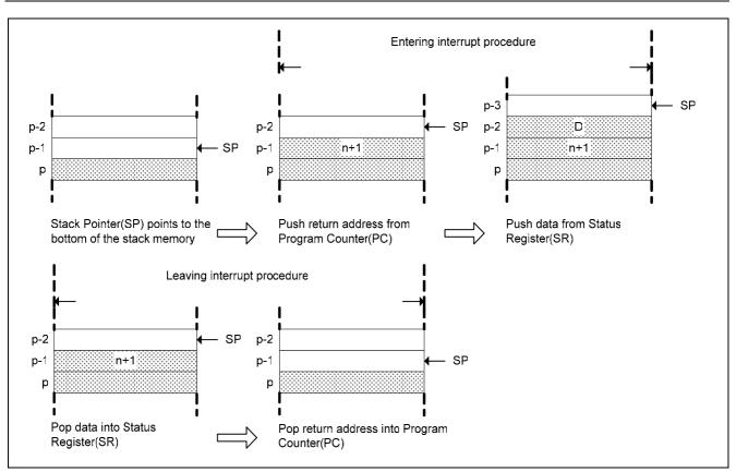
Figure 5-12 Stack memory operation with interrupt procedure
