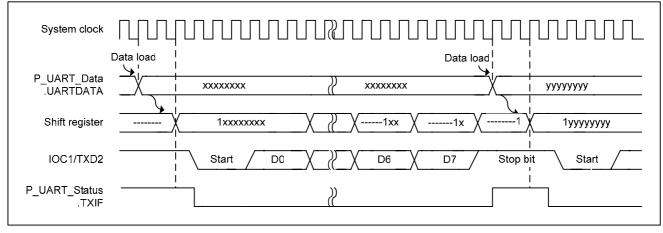
Figure 5-77 Data Transmission Timing
