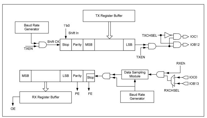
Figure 5-75 UART block diagram
