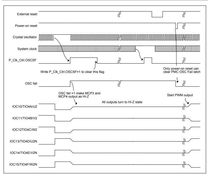
Figure 5-67 Oscillator stopped timing
