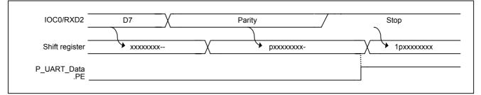
Figure 5-81 Parity Error timing
