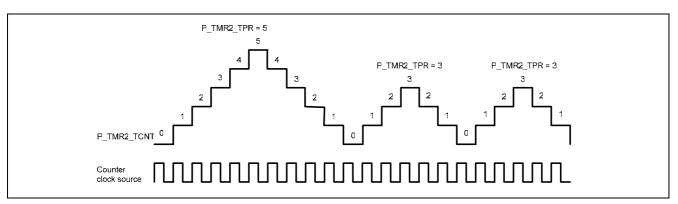
Figure 5-48 Continuous up/down counting example (CCLS = 111'b, CKEGS = 00'b, TMRPS = 000'b)
