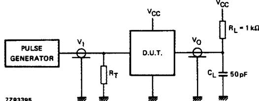
Fig.7 Test circuit (open drain)
