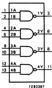
Fig.4 Functional diagram.
