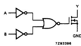
Fig.5 Logic diagram (one gate).
