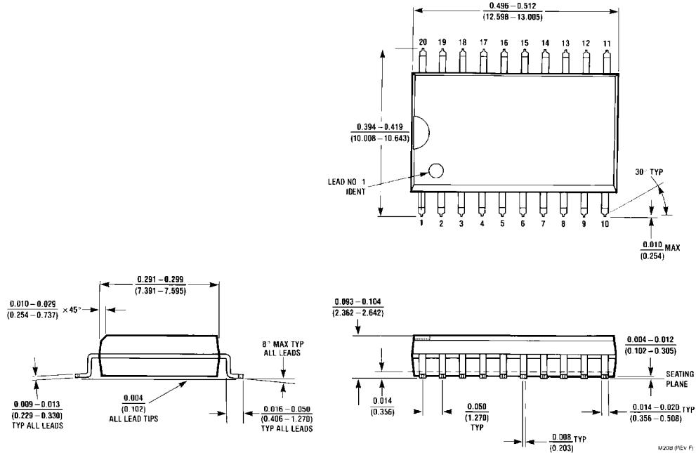
20-Lead Small Outline Integrated Circuit (SOIC), JEDEC MS-013, 0.300" Wide
