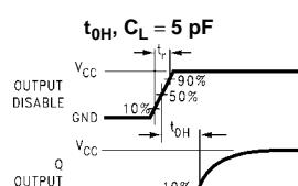
$t_{H0}, C_L = 5 \text{ pF}$
