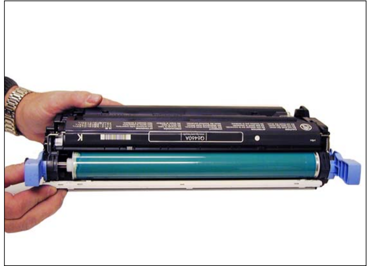
46. Check to make sure the drum cover closes properly.
