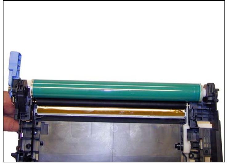
21. Install the drum in the cartridge, large hub side to the NON contact side.
