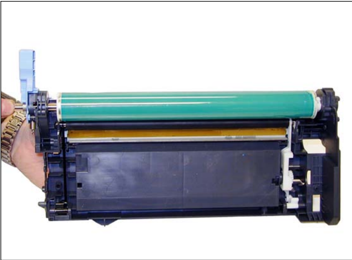
22. Slide the drum axle in from the contact side. Make sure you do not damage the copper drum contacts. Both tabs must be in contact with the axle.
