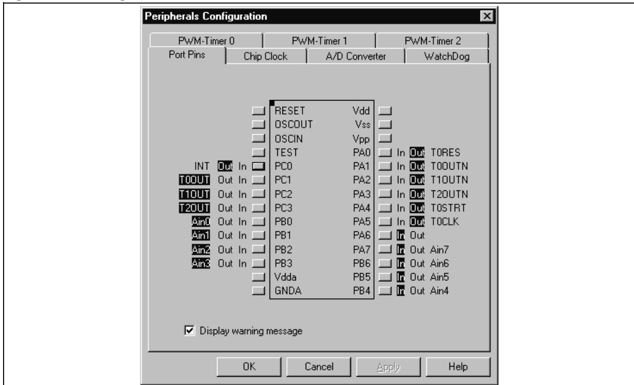
AD converter is configured with four channels, which are converted continually: Ain0 and Ain1 are used to detect ZCa and ZCb; Ain2 is used to convert the information coming from Rsense that is related with the overall maximum current; Ain3 is used to convert the voltage coming from the potentiometer that sets the target speed.
