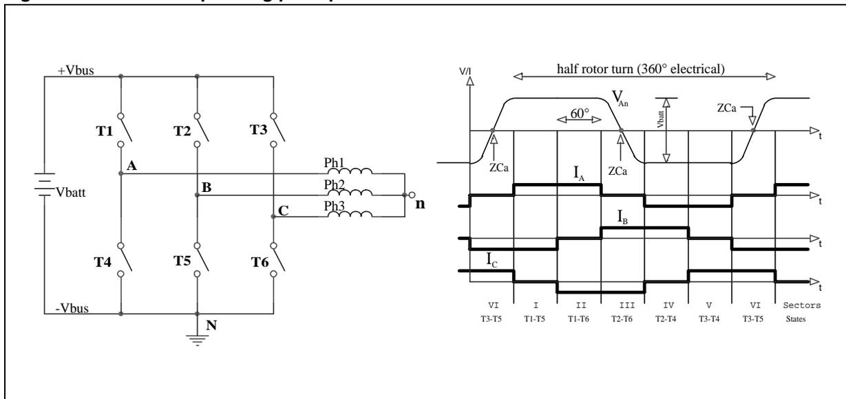
The name "six-steps" arises from the finite time-steps in which the whole period  $0 \div 2\pi$  can be shared. Being our motor a two pole pairs, the electrical period  $0 \div 2\pi$  represents half turn of the rotor.
