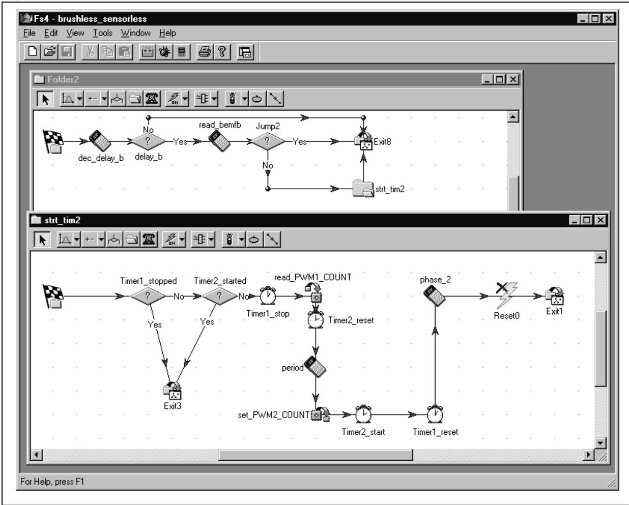
The timers tasks described above allow to synchronize each BEMF zero-crossing with the rising/falling-edge of Timer2. Then the Timer2 edge events to control the commutation of the driver signals to be sent to Port A. Since Timer1 starts and stops on two BEMF events, its content also gives information about the rotor speed to implement the PID fuzzy controller.
