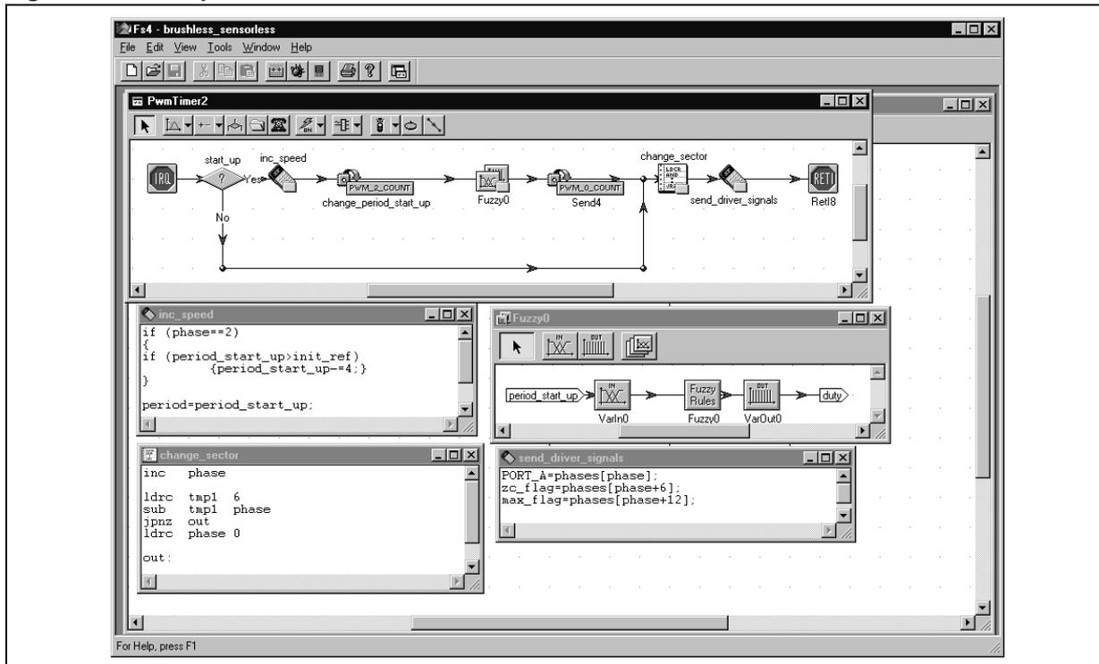
This pattern is available in a look-up table stored in the ST52 x420 EPROM. Since the Timer2 subroutine is executed at each T/6 period then PORT\_A will change its pattern at each T/6. The following figure shows the pattern for the driver topology previously discussed.
