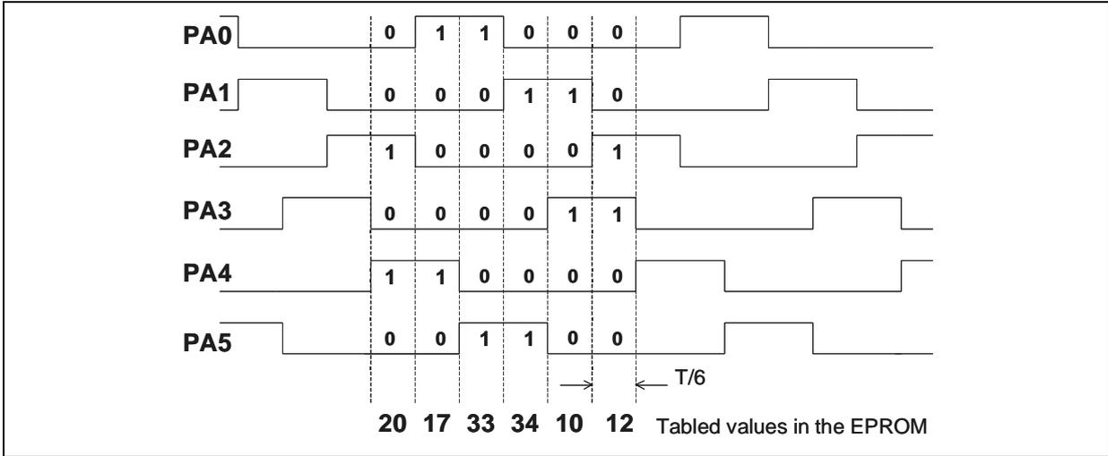
The same look-up table is used to store some flags that are addressed during the variable's status change. These flags are used to indicate to the AD interrupt routine the task to be performed in that moment (find max, find ZCa or ZCb) accordingly to the related sector.
