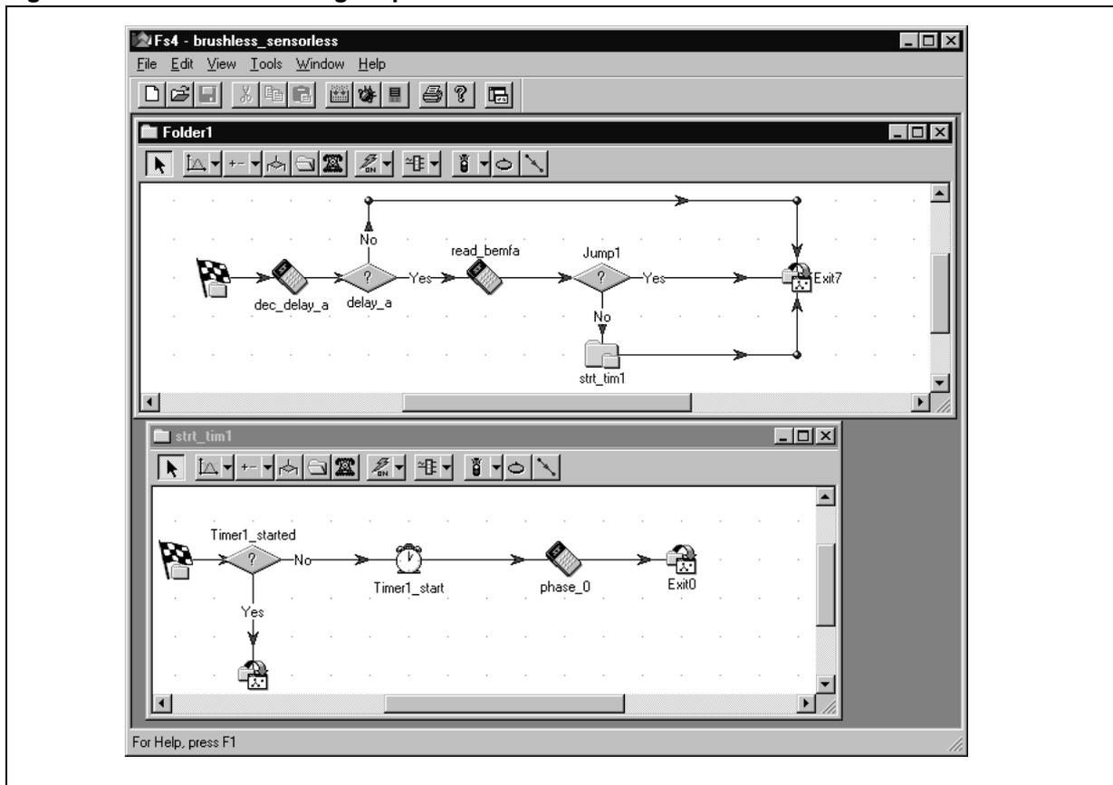
The blocks 'dec\_delay\_a' and 'delay\_a' implement a blanking time necessary to avoid the sampling of commutation spike. This spike arises from the coil opening in correspondence to the switching sector (See technical literature for further reference).
