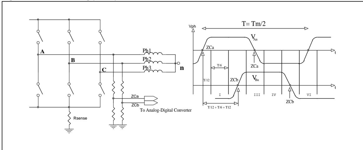
Only two phases are monitored in order to detect their zero-crossing. In fact, only two temporal information are enough to know position and speed of the rotor with enough accuracy.
