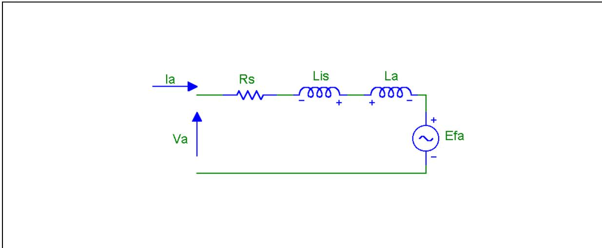
$E_{fa}$  represents the Back-EMF (bemf). This is the voltage that the permanent magnet rotor induces in the stator coil when motion takes place. This EMF is always present during the normal driving of the motor and opposes a counter-force to the motion of the shaft that is proportional to the rotor speed.
