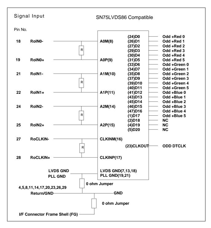
The module uses a 100ohm resistor between positive and negative lines of each receiver input.
