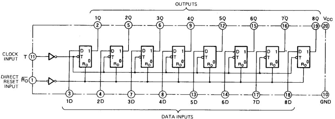
**OCTAL POSITIVE EDGE-TRIGGERED D-TYPE FLIP FLOP WITH RESET**
