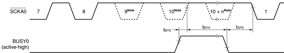
**Note**  $\overline{SCKA0}$  does not become low level here, but the timing is illustrated so that the timing specifications can be shown.
