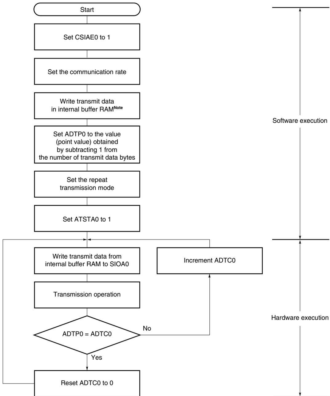
CSIAE0: Bit 7 of serial operation mode specification register 0 (CSIMA0)
