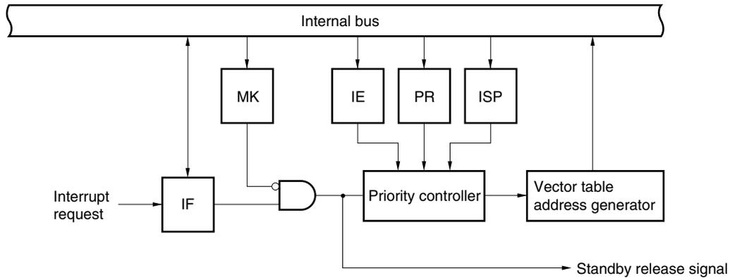
(B) External maskable interrupt (INTP0 to INTP7)
