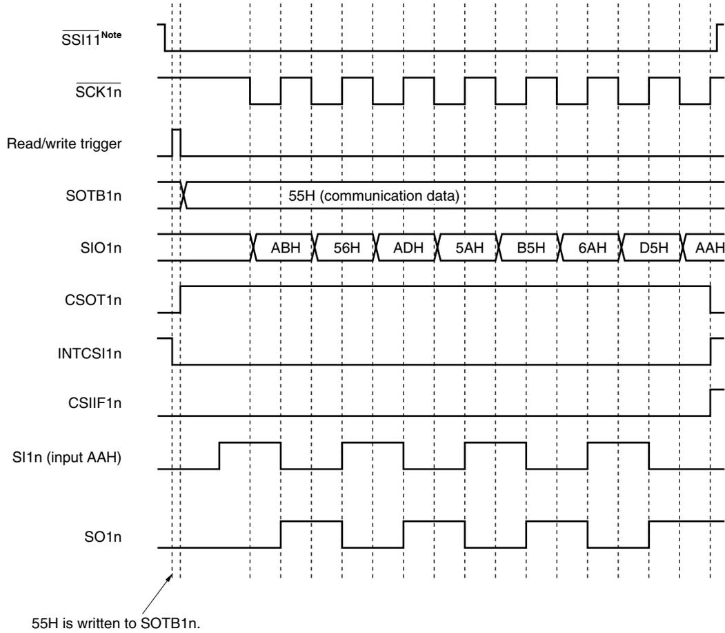
**Note** The SSE11 flag and  $\overline{\text{SSI11}}$  pin are available only for serial interface CSI11, and are used in the slave mode.
