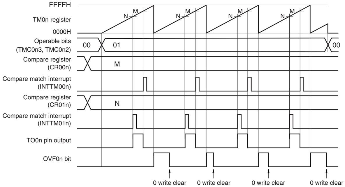
This is an application example where two compare registers are used in the free-running timer mode. The output level of the TO0n pin is reversed each time the count value of TM0n matches the set value of CR00n or CR01n. When the count value matches the register value, the INTTM00n or INTTM01n signal is generated.
