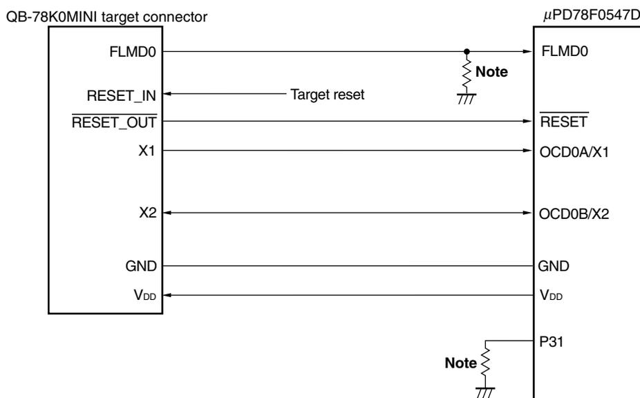
**Note** Make pull-down resistor 470  $\Omega$  or more (10 k $\Omega$ : recommended).
