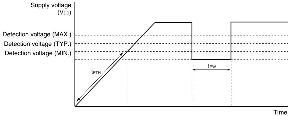
Supply Voltage Rise Time ( $T_A = -40$  to  $+85^\circ\text{C}$ ,  $V_{SS} = EV_{SS} = 0$  V)
