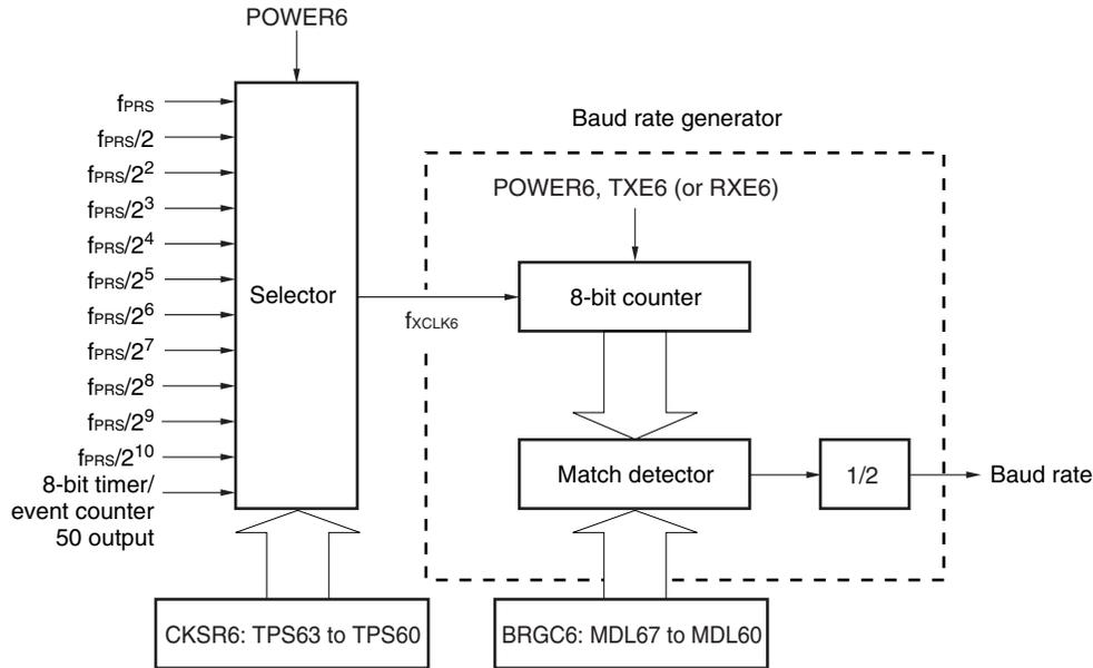
**Remark** POWER6: Bit 7 of asynchronous serial interface operation mode register 6 (ASIM6)
