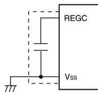
**Caution** Keep the wiring length as short as possible for the broken-line part in the above figure.
