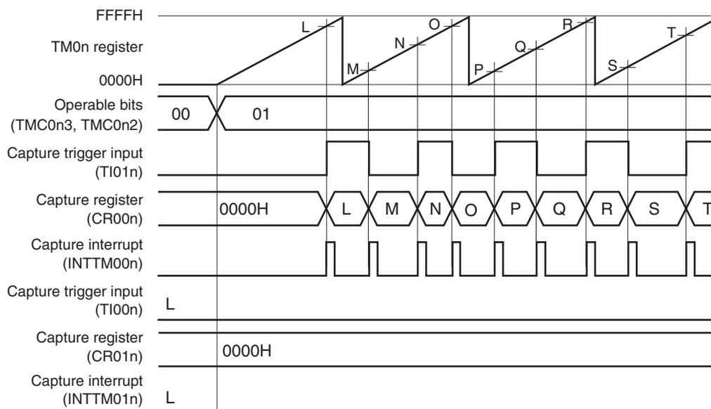
This is an application example where both the edges of the TI01n pin are detected and the count value is captured to CR00n in the free-running timer mode.
