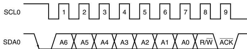
When the local address is received,  $\overline{\text{ACK}}$  is automatically generated, regardless of the value of ACEK0. When an address other than that of the local address is received,  $\overline{\text{ACK}}$  is not generated (NACK).
