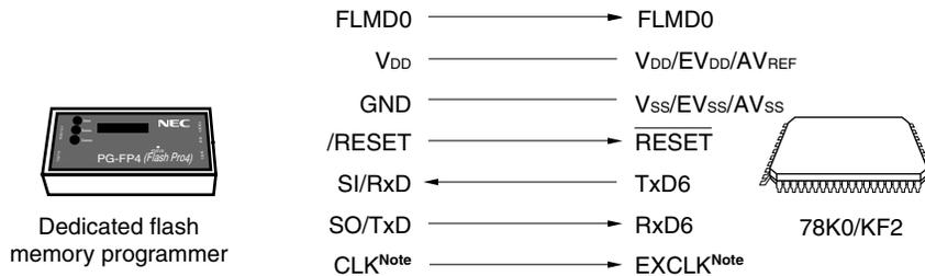
**Note** The above figure illustrates an example of wiring when using the clock output from the PG-FP4 or FL-PR4. When using the clock output from the PG-FPL3 or FP-LITE3, connect CLK to X1/P121 (pin 15), and connect its inverted signal to X2/EXCLK/P122 (pin 14).
