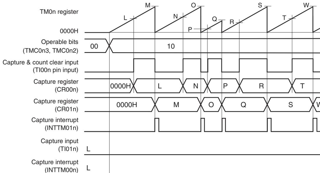
This is an application example where the pulse width of the signal input to the TI00n pin is measured.
