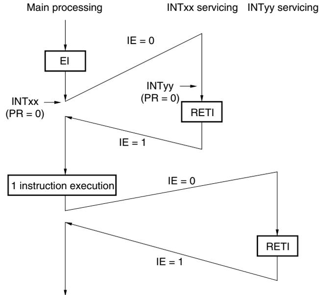
Interrupts are not enabled during servicing of interrupt INTxx (EI instruction is not issued), therefore, interrupt request INTyy is not acknowledged and multiple interrupt servicing does not take place. The INTyy interrupt request is held pending, and is acknowledged following execution of one main processing instruction.
