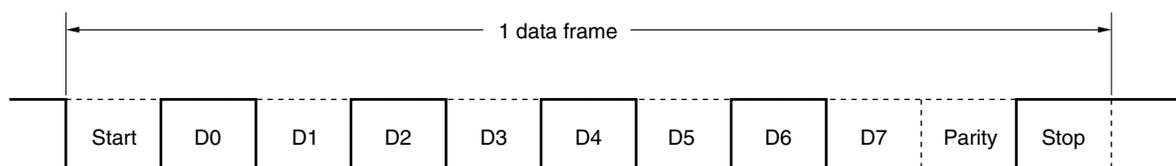
**2. Data length: 7 bits, Parity: Odd parity, Stop bit: 2 bits, Communication data: 36H**
