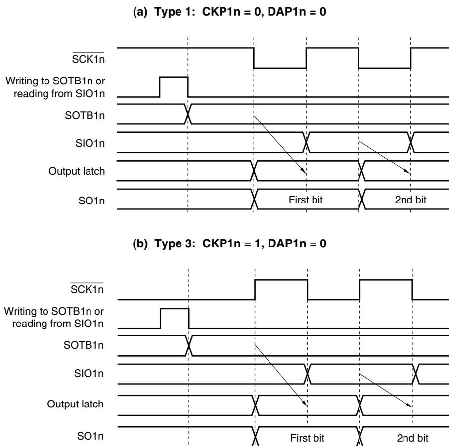
The first bit is directly latched by the SOTB1n register to the output latch at the falling (or rising) edge of  $\overline{SCK1n}$ , and output from the SO1n pin via an output selector. Then, the value of the SOTB1n register is transferred to the SIO1n register at the next rising (or falling) edge of  $\overline{SCK1n}$ , and shifted one bit. At the same time, the first bit of the receive data is stored in the SIO1n register via the SI1n pin.
