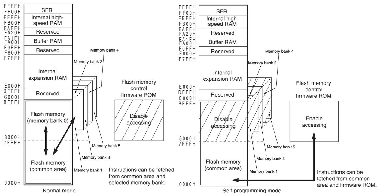
The following figure illustrates a flow of rewriting the flash memory by using a self programming sample library.
