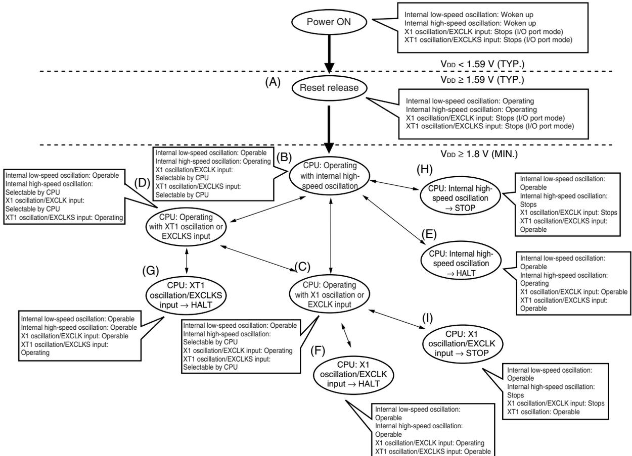
**Remark** In the 2.7 V/1.59 V POC mode (option byte: POCMODE = 1), the CPU clock status changes to (A) in the above figure when the supply voltage exceeds 2.7 V (TYP.), and to (B) after reset processing (11 to 45  $\mu\text{s}$ ).
