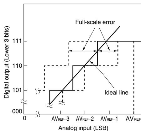
**Figure 13-18. Integral Linearity Error**
