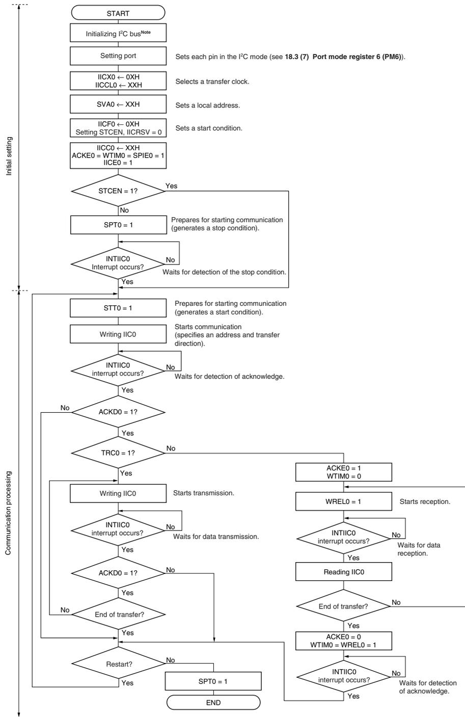
**Note** Release (SCL0 and SDA0 pins = high level) the I<sup>2</sup>C bus in conformance with the specifications of the product that is communicating. If EEPROM is outputting a low level to the SDA0 pin, for example, set the SCL0 pin in the output port mode, and output a clock pulse from the output port until the SDA0 pin is constantly at high level.
