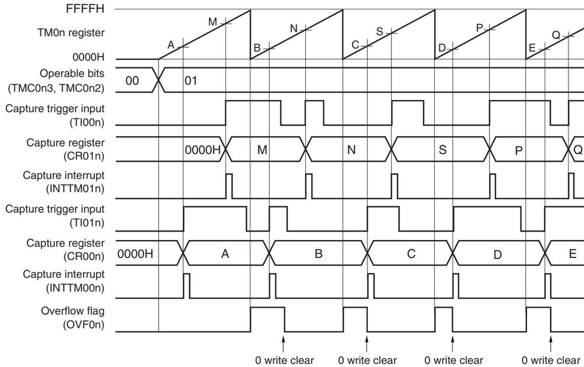
This is an application example where the count values that have been captured at the valid edges of separate capture trigger signals are stored in separate capture registers in the free-running timer mode.
