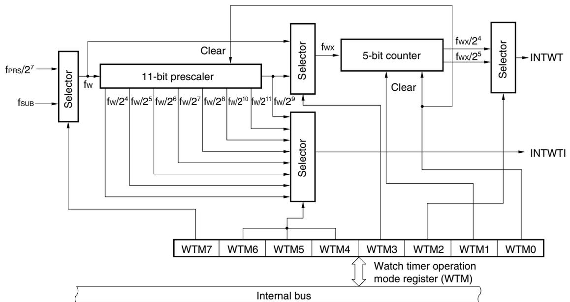
**Remark**  $f_{PRS}$ : Peripheral hardware clock frequency
