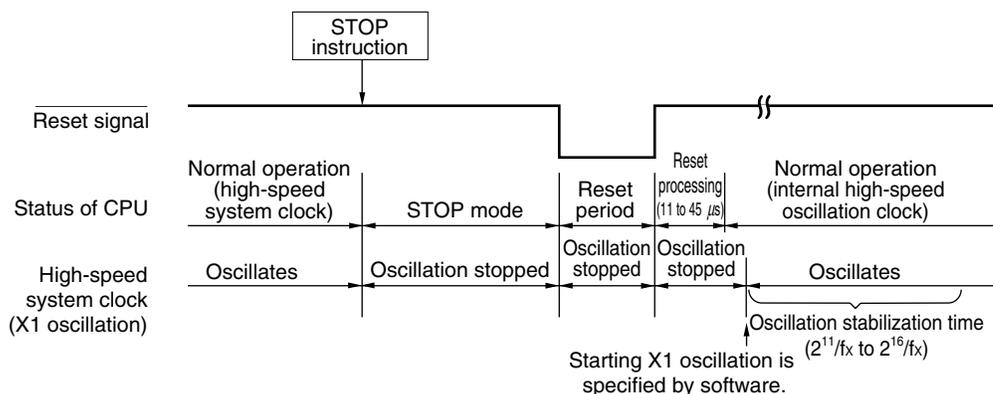
**(2) When internal high-speed oscillation clock is used as CPU clock**
