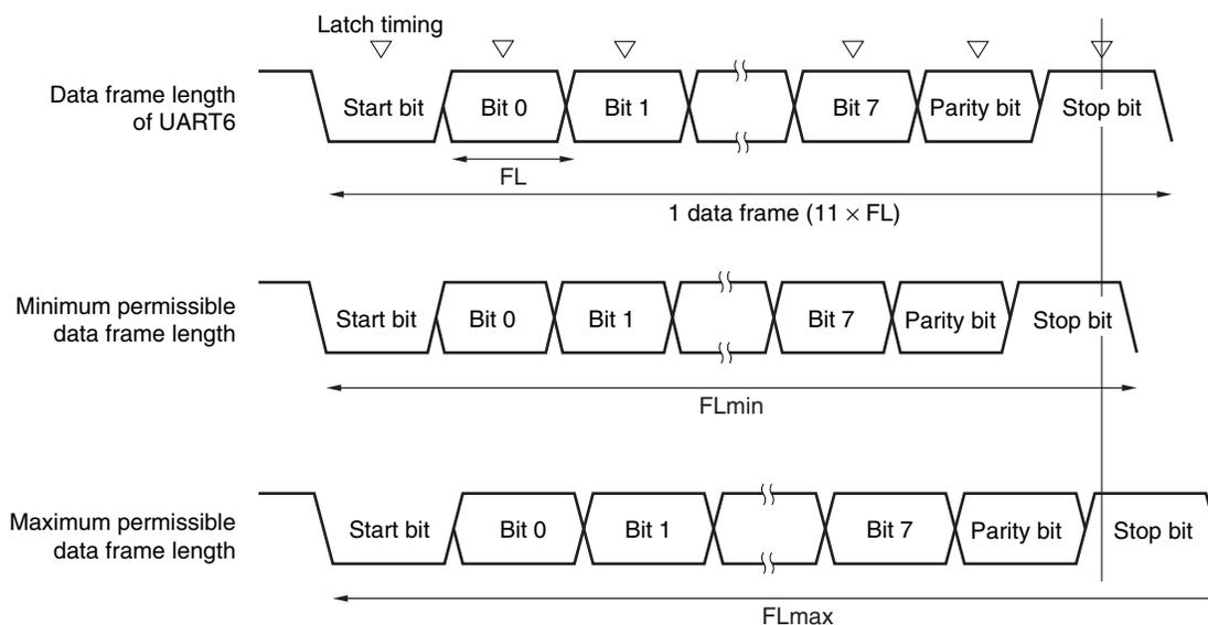
As shown in Figure 15-25, the latch timing of the receive data is determined by the counter set by baud rate generator control register 6 (BRGC6) after the start bit has been detected. If the last data (stop bit) meets this latch timing, the data can be correctly received.
