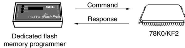
The flash memory control commands of the 78K0/KF2 are listed in the table below. All these commands are issued from the programmer and the 78K0/KF2 perform processing corresponding to the respective commands.
