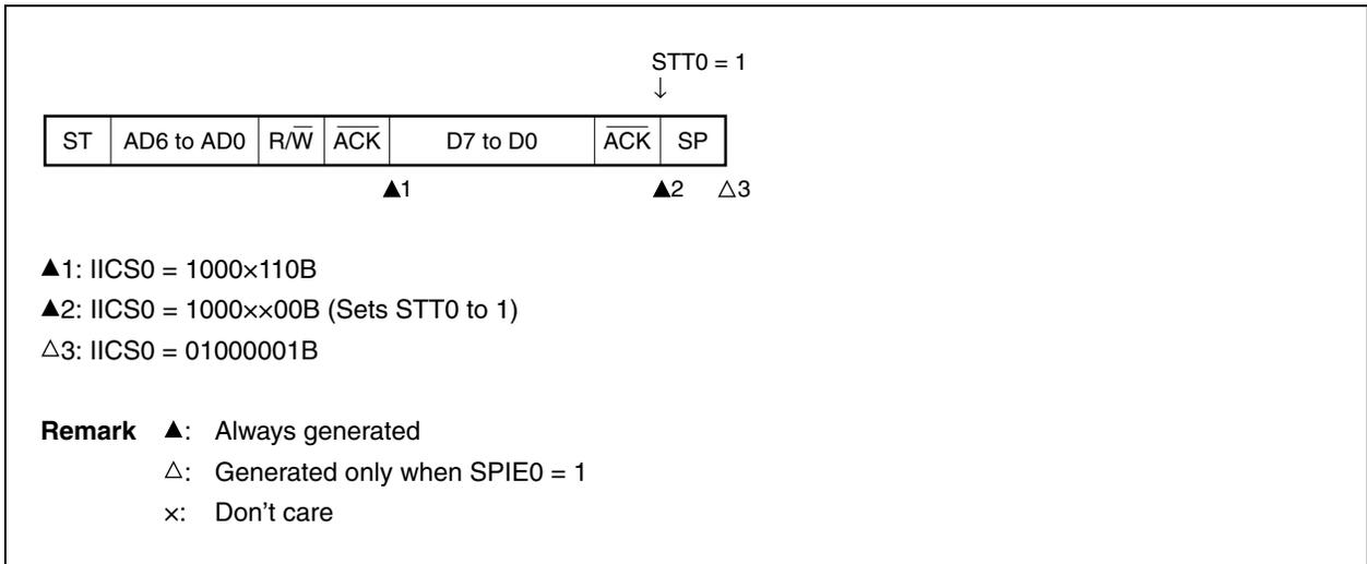
**(h) When arbitration loss occurs due to low-level data when attempting to generate a stop condition****(i) When WTIM0 = 0**
