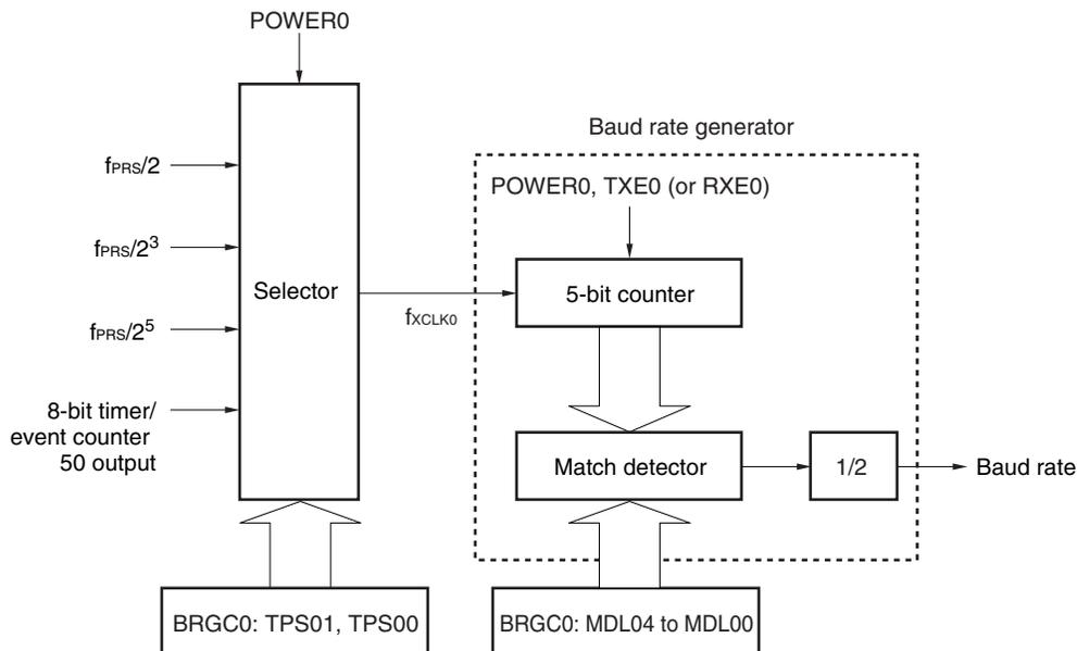
**Remark** POWER0: Bit 7 of asynchronous serial interface operation mode register 0 (ASIM0)
