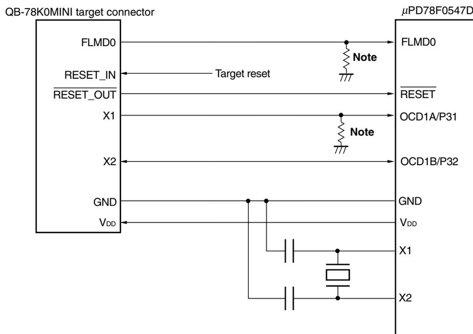
**Note** Make pull-down resistor 470  $\Omega$  or more (10 k $\Omega$ : recommended).
