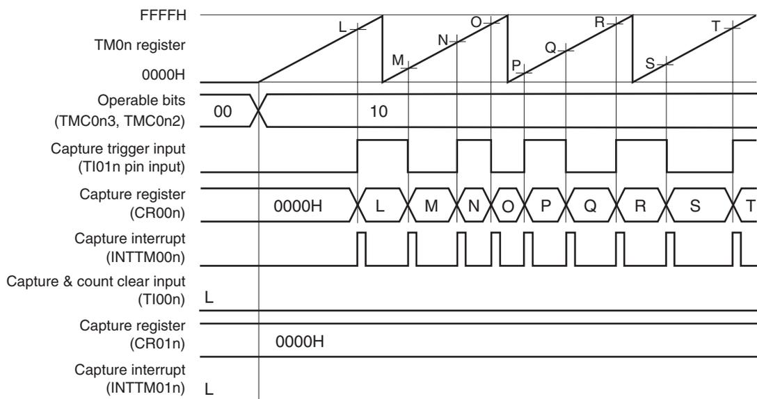
This is a timing example where an edge is not input to the TI00n pin, in an application where the count value is captured to CR00n when the rising or falling edge of the TI01n pin is detected.
