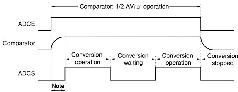
**Note** To stabilize the internal circuit, the time from the rising of the ADCE bit to the falling of the ADCS bit must be  $1\ \mu\text{s}$  or longer.
