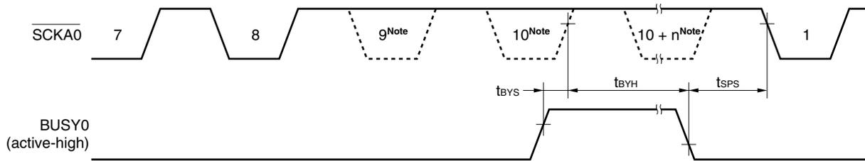
**Note**  $\overline{SCKA0}$  does not become low level here, but the timing is illustrated so that the timing specifications can be shown.
