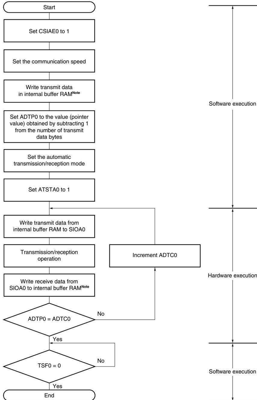
CSIAE0: Bit 7 of serial operation mode specification register 0 (CSIMA0)
