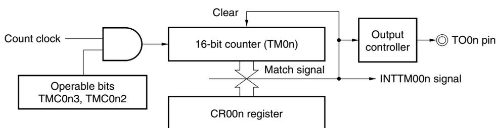
**Figure 7-21. Basic Timing Example of Square-Wave Output Operation**
