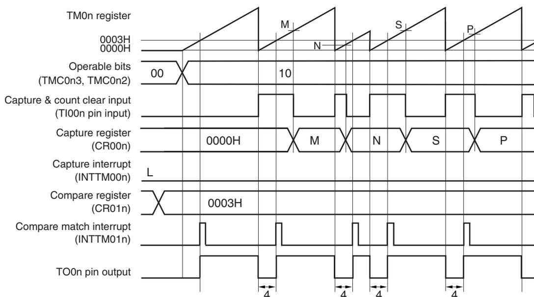
This is an application example where the width set to CR01n (4 clocks in this example) is to be output from the TO0n pin when the count value has been captured & cleared.
