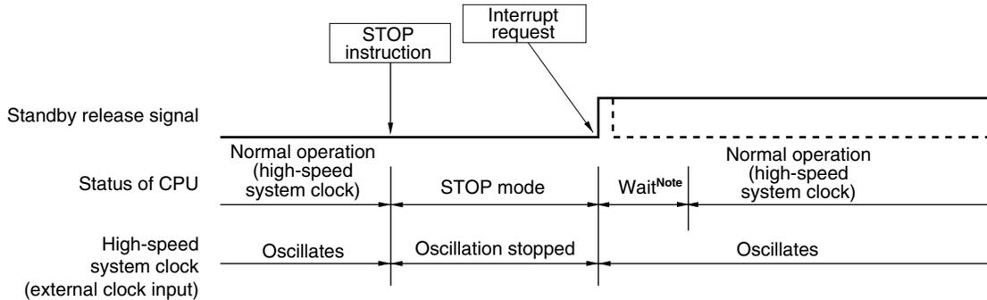
(3) When internal high-speed oscillation clock is used as CPU clock
