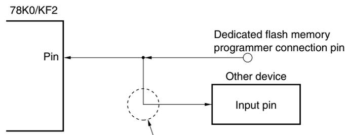
If the signal output by the dedicated flash memory programmer in the flash memory programming mode affects the other device, isolate the signal of the other device.
