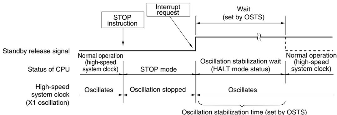
(2) When high-speed system clock (external clock input) is used as CPU clock (1/2)
