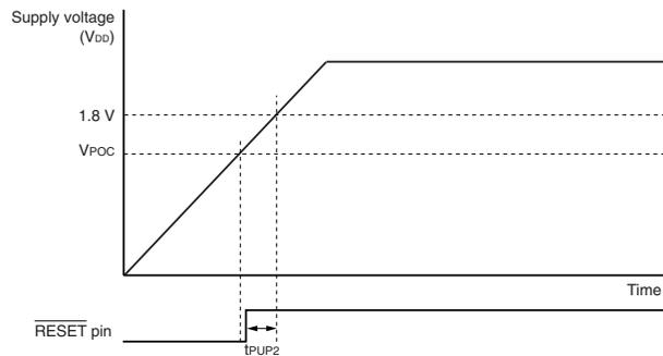
**2.7 V POC Circuit Characteristics ( $T_A = -40$  to  $+85^\circ\text{C}$ ,  $V_{SS} = EV_{SS} = 0$  V)**
