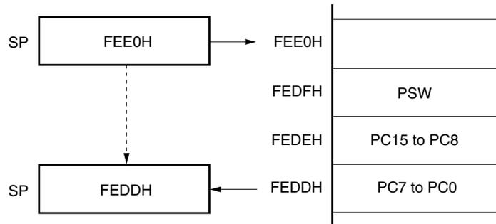
Figure 3-14. Data to Be Restored from Stack Memory
