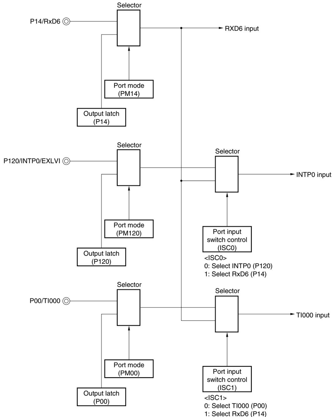
**Remark** ISC0, ISC1: Bits 0 and 1 of the input switch control register (ISC) (see **Figure 15-11**)
