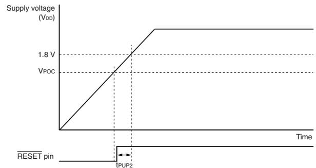
2.7 V POC Circuit Characteristics ( $T_A = -40$  to  $+85^\circ\text{C}$ ,  $V_{SS} = EV_{SS} = 0$  V)
