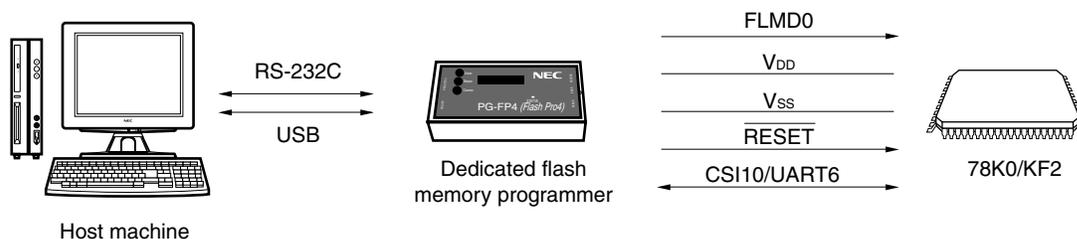
A host machine that controls the dedicated flash memory programmer is necessary.
