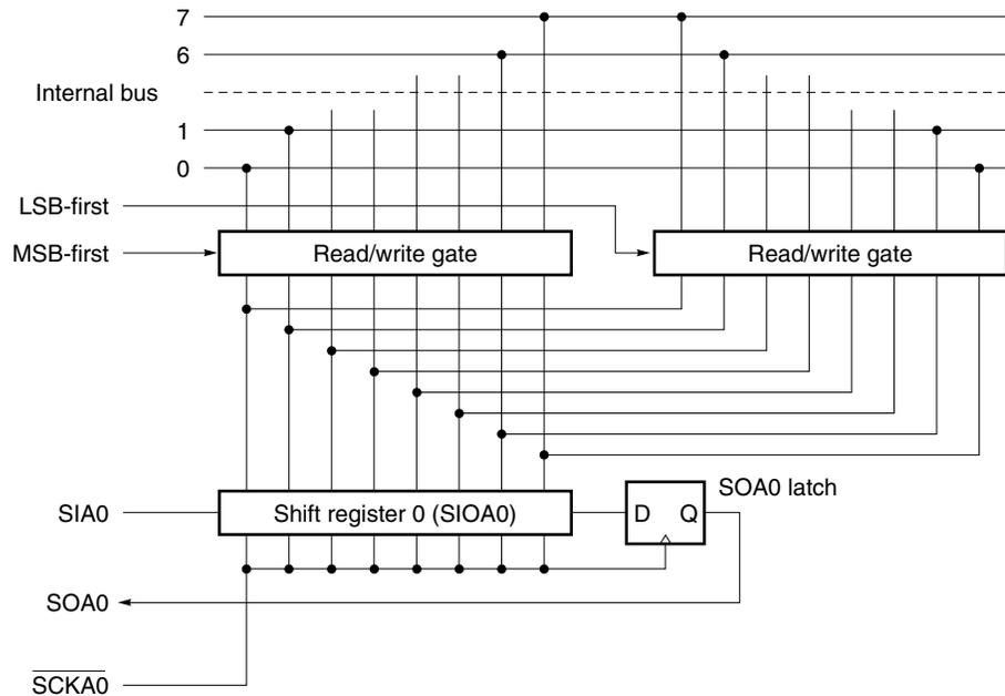
Start bit switching is realized by switching the bit order for data written to SIOA0. The SIOA0 shift order remains unchanged.
