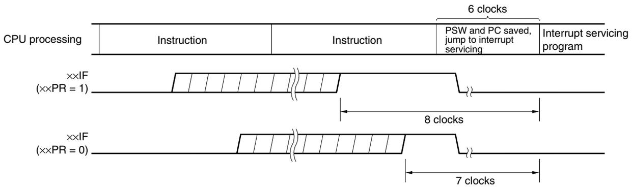
**Remark** 1 clock: 1/f<sub>CPU</sub> (f<sub>CPU</sub>: CPU clock)
