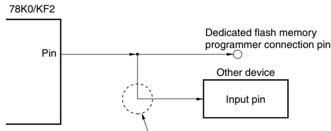
If the signal output by the 78K0/KF2 in the flash memory programming mode affects the other device, isolate the signal of the other device.
