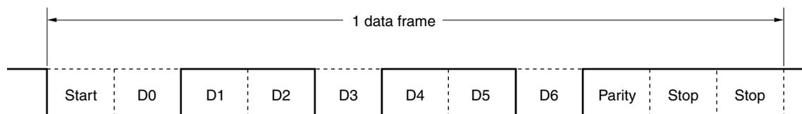
5. Data length: 8 bits, LSB first, Parity: None, Stop bit: 1 bit, Communication data: 87H
