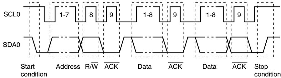
The master device generates the start condition, slave address, and stop condition. The acknowledge ( $\overline{\text{ACK}}$ ) can be generated by either the master or slave device (normally, it is output by the device that receives 8-bit data).
