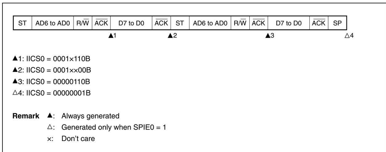
**(3) Slave device operation (when receiving extension code)**
