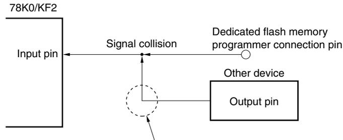
In the flash memory programming mode, the signal output by the device collides with the signal sent from the dedicated flash programmer. Therefore, isolate the signal of the other device.
