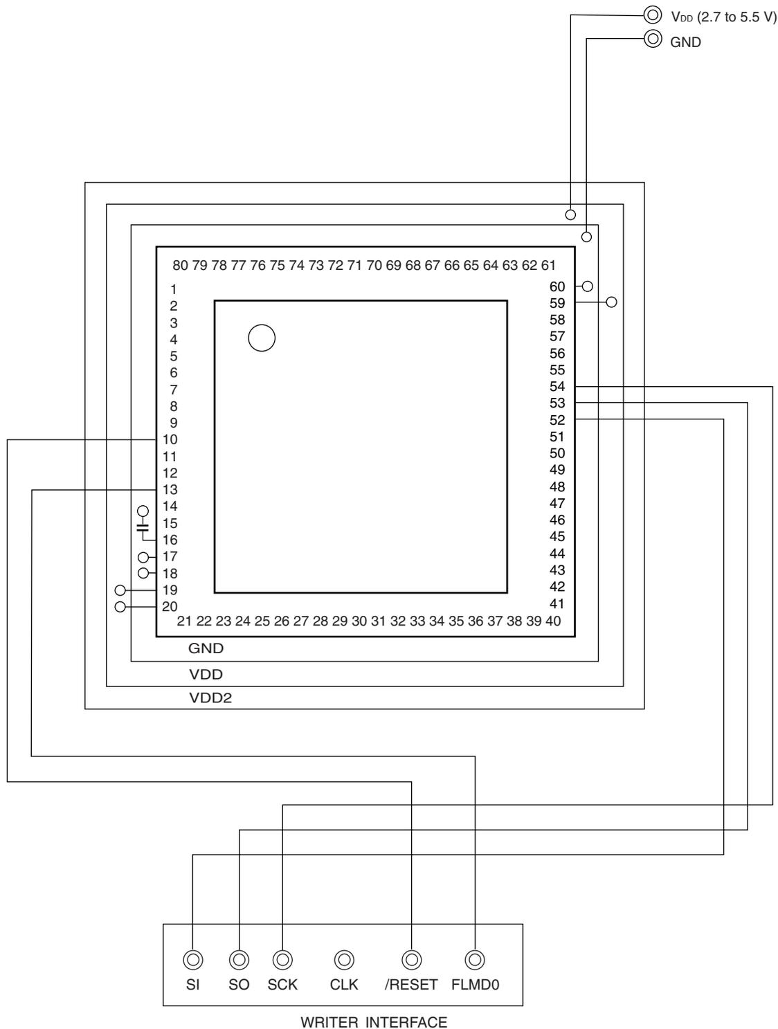
Figure 27-4. Example of Wiring Adapter for Flash Memory Writing in UART (UART6) Mode
