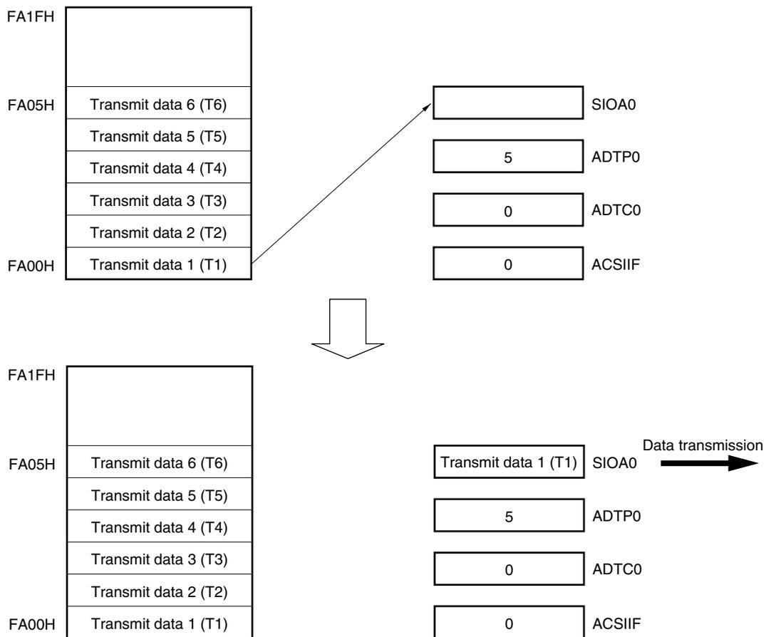
**Figure 17-15. Internal Buffer RAM Operation in Automatic Transmission/Reception Mode (Starting Transmission/Reception) (2/2)**
