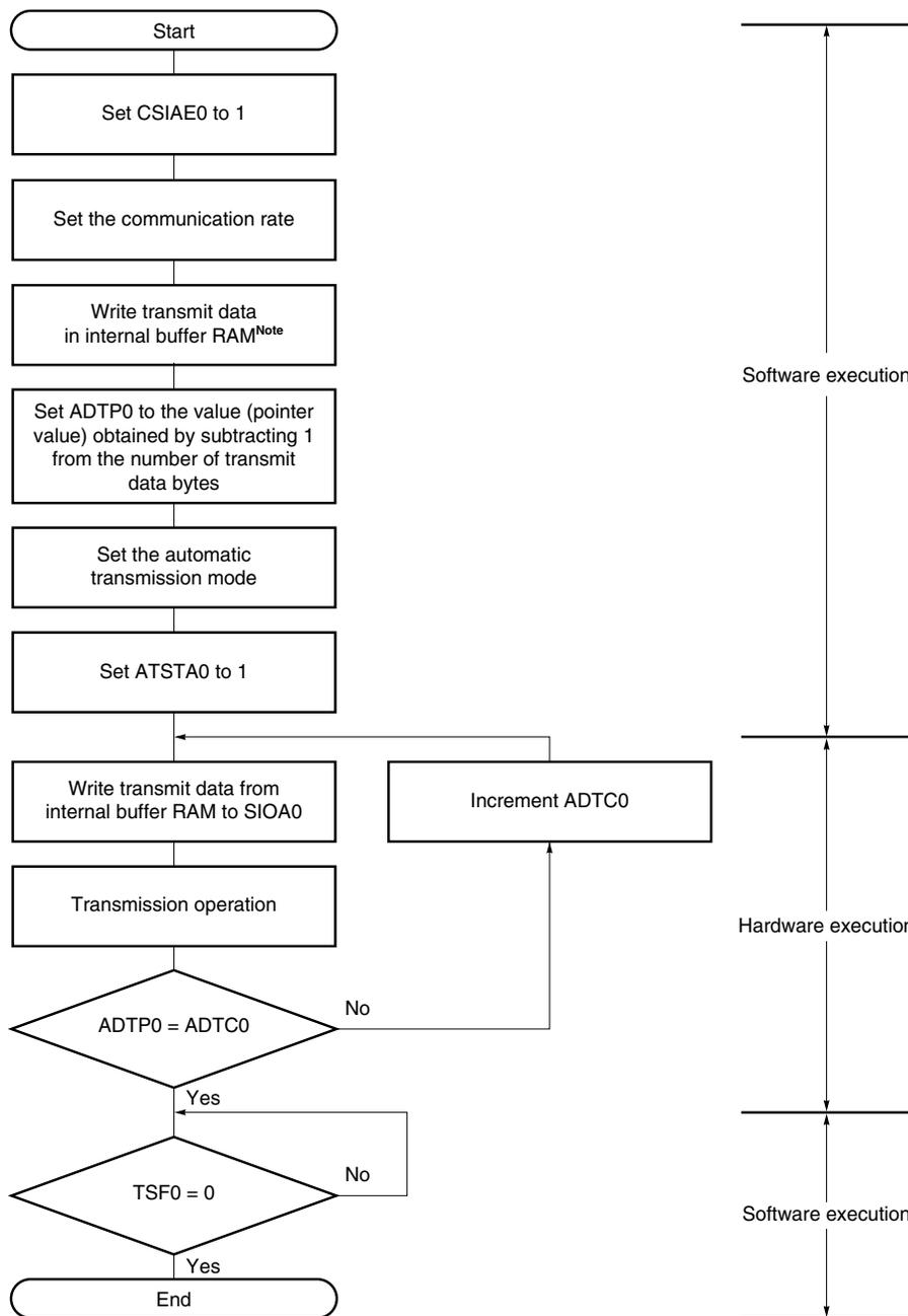
CSIAE0: Bit 7 of serial operation mode specification register 0 (CSIMA0)
