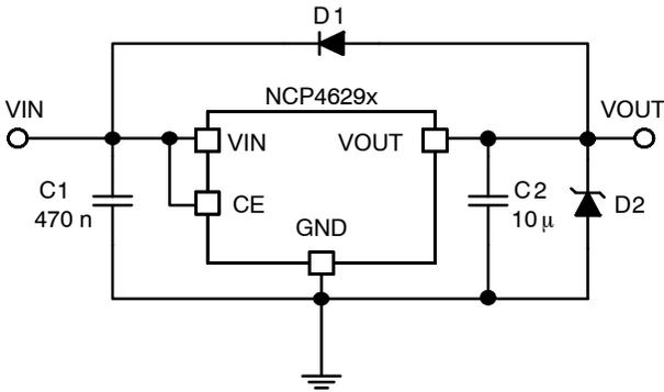
Figure 4. Typical Application Schematic with Protective Diodes
