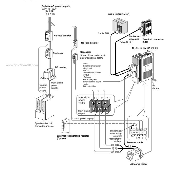
When the power supply is shared with converter, if the total current capacity is over 60A, set up a no fuse breaker and contactor for the main circuit power supply for SVJ2 separately.
