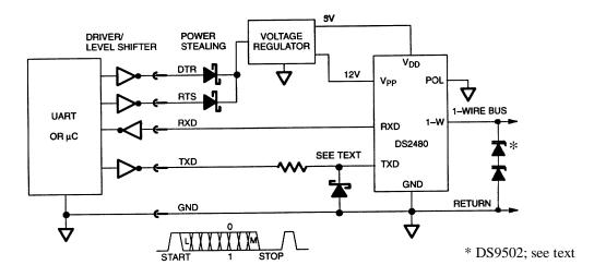
The signals DTR and RTS provide the power to operate the DS2480B. The resistor in the TXD line and the Schottky diode limit the negative voltage at the TXD pin of the DS2480B to 0.3V maximum. The resistor is typically 4.7 k $\Omega$ . If the inverting driver is current–limited to 1 mA the resistor is not required.
