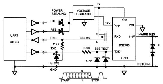
\* DS9502; only one device needed for 5V operation
