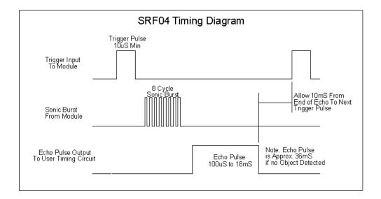
The SRF04 outputs a high-going pulse that corresponds to time required for the echo to return. **RCTIME** (for the BS2 and BS2e) and **PULSIN** (for the BS2sx, BS2p, and BS2pe) can be used to measure it and determine the distance to the target. Using **RCTIME** on the BS2 and BS2e allows us to measure the echo
