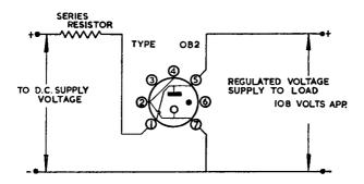
TYPICAL CIRCUIT TO PROVIDE A REGULATED SUPPLY VOLTAGE. REMOVAL OF THE VALVE FROM THE SOCKET DISCONNECTS THE VOLTAGE FROM THE LOAD
