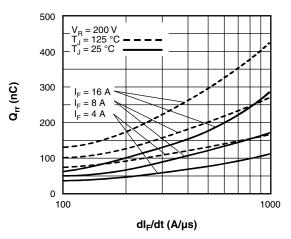
Fig. 7 - Typical Stored Charge vs. dl<sub>F</sub>/dt
