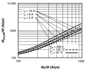
Fig. 8 - Typical dl<sub>(rec)M</sub>/dt vs. dl<sub>F</sub>/dt
