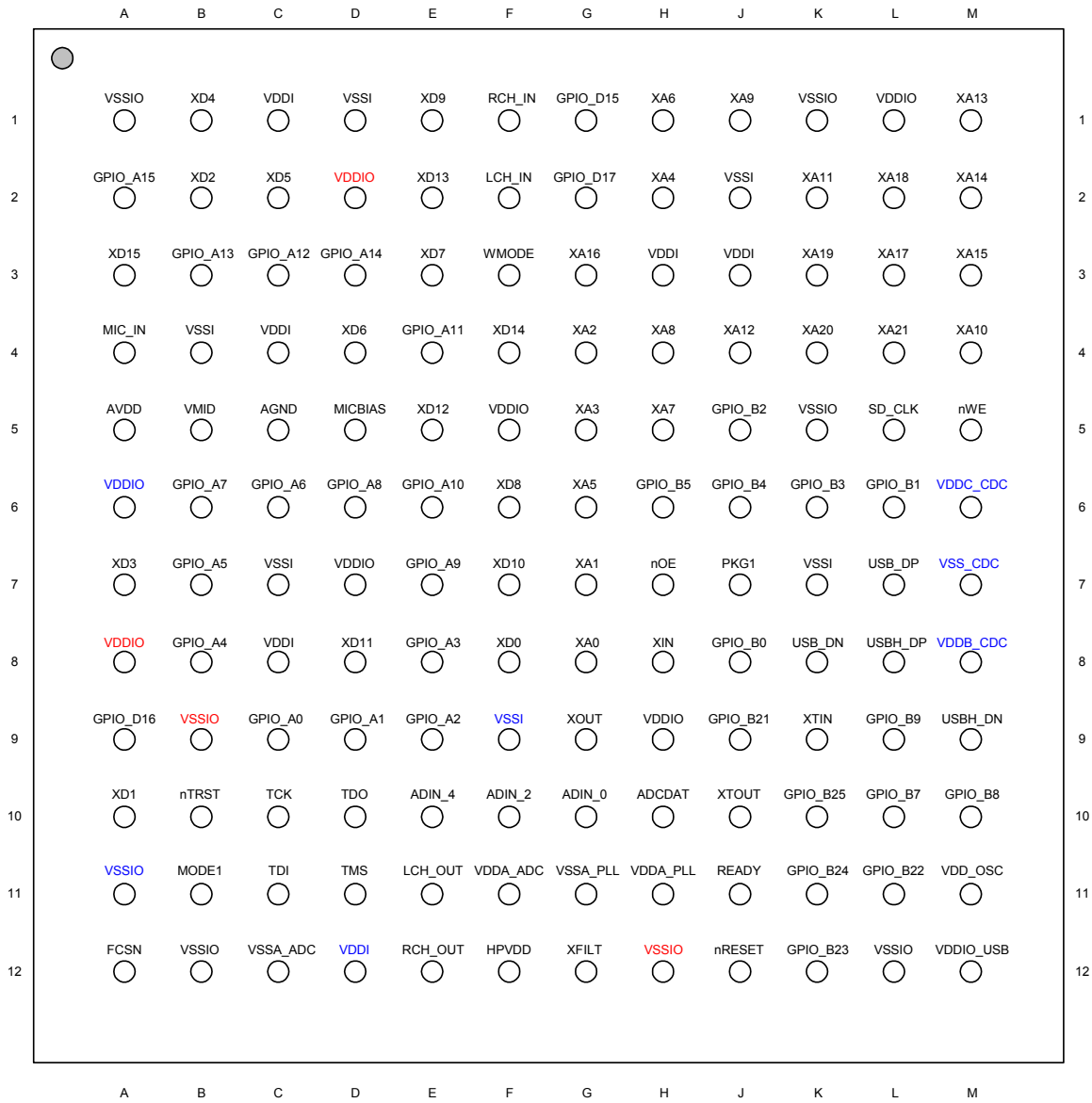
Figure 1.14 TCC768 Package Diagram (144-BGA-1010 / Bottom View)
