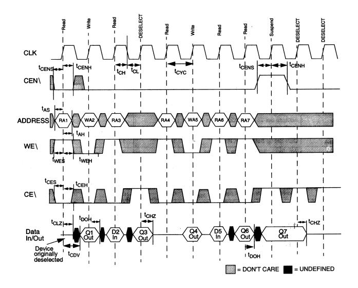
WE\ is the combination of WE\ & BWSx\ (x=a, b, c, d) to define a write cycle (see Write Cycle Description table). CE\ is the combination of CE1\, CE2, and CE3\. All chip selects need to be active in order to select the device. Any chip select can deselect the device. RAx stands for Read Address X, WA stands for Write Address X, Dx stands for Data-in X, Qx stands for Data-out X.
