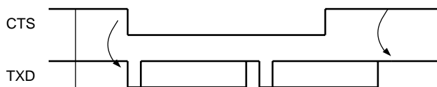
Figure 20-17. Transmitter Behavior when Operating with Hardware Handshaking
