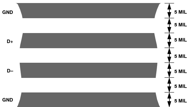
Figure 22. Typical Arrangement of Signal Tracks
