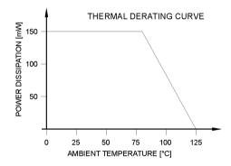
Figure 1: Maximum power dissipation with respect to temperature
