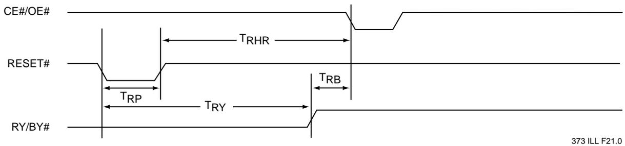
FIGURE 16: RESET# TIMING DIAGRAM
