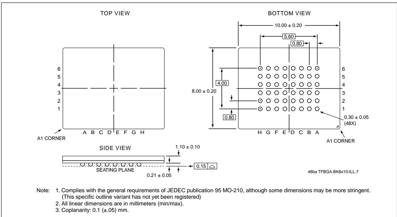
48-BALL THIN PROFILE FINE-PITCH BALL GRID ARRAY (TFBGA) 8MM X 10MM
