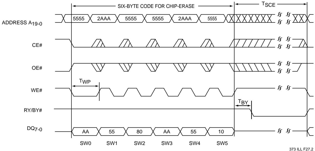
Note: This device also supports CE# controlled Chip-Erase operation. The WE# and CE# signals are interchangeable as long as minimum timings are met. (See Table 13)
