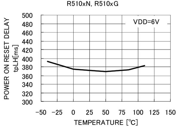
9) Detector Output Delay Time vs. Temperature
